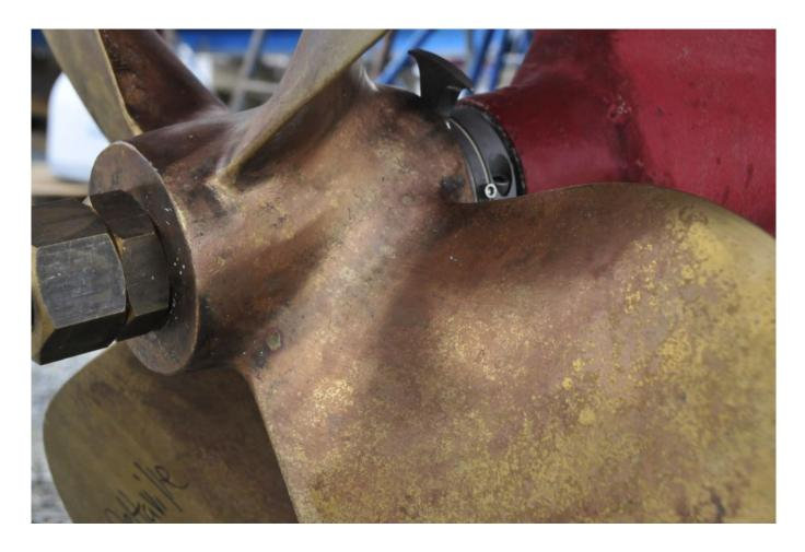
If not properly cathodically protected, manganese bronze propellers are susceptible to a type of corrosion referred to as dezincification. The telltale pinkish hue is an indication that this prop is suffering from this phenomenon.
