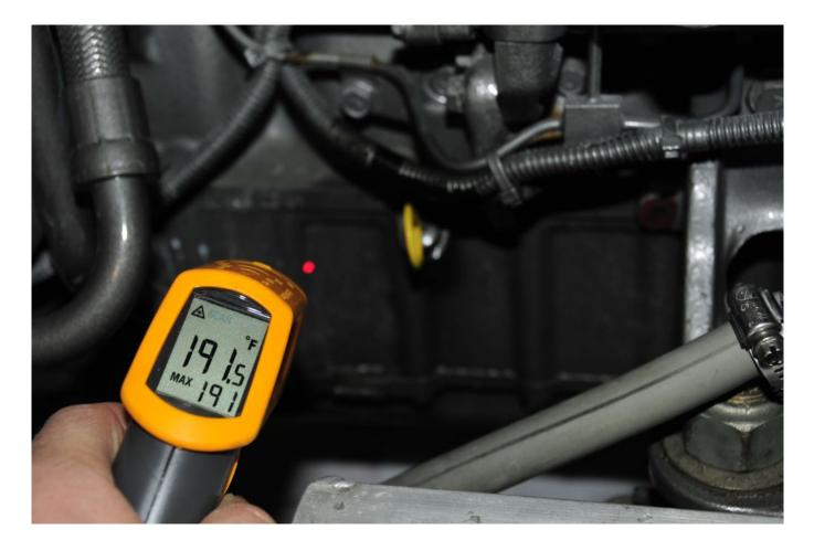
Oil temperature is most accurately measured, using an infrared pyrometer, at the vertical center of the side of the oil pan.
