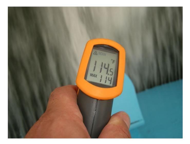
Infrared pyrometers can be used to accurately measure the temperature of liquid, including seawater.
