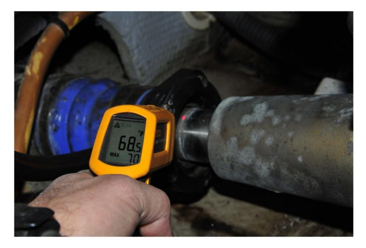
Monitoring stuffing box temperature is critical, it's the only true means of determining if it's working properly. When doing so, be sure not to measure the shaft which, being reflective it will skew the readings.
