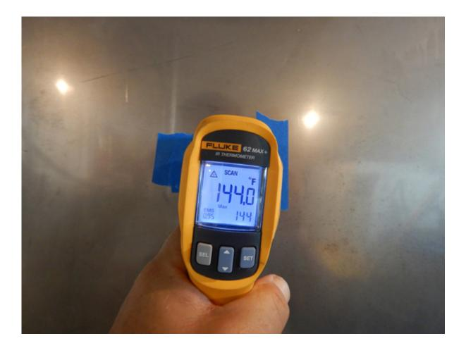
As versatile and accurate as IR pyrometers are, they can be fooled by highly reflective surfaces like stainless steel, chrome and even reflective insulation, with a resultant inaccurate reading that is typically lower than that of the actual temperature. This can be overcome by applying dark or non reflective paint or tape to the surface that is being measured.
