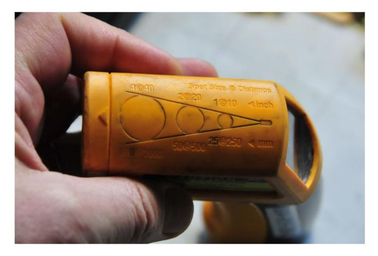
The measurement "footprint" of an IR pyrometer is cone shaped, and thus the farther the gun is from the surface being measured, the larger the measurement area, and the lower the accuracy if the temperature within that area varies. Therefore, it is advisable to place the gun as close to the surface being measured as is safely possible.
