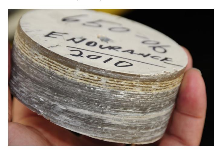
Each laminate is a separate layer of fabric and resin, which looks somewhat like tree rings when section cut. The one shown here includes four layers of Kevlar.
