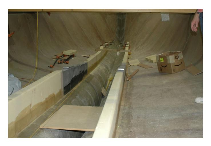
Stringers, shaft logs and other structure components, utilize secondary bonds.
