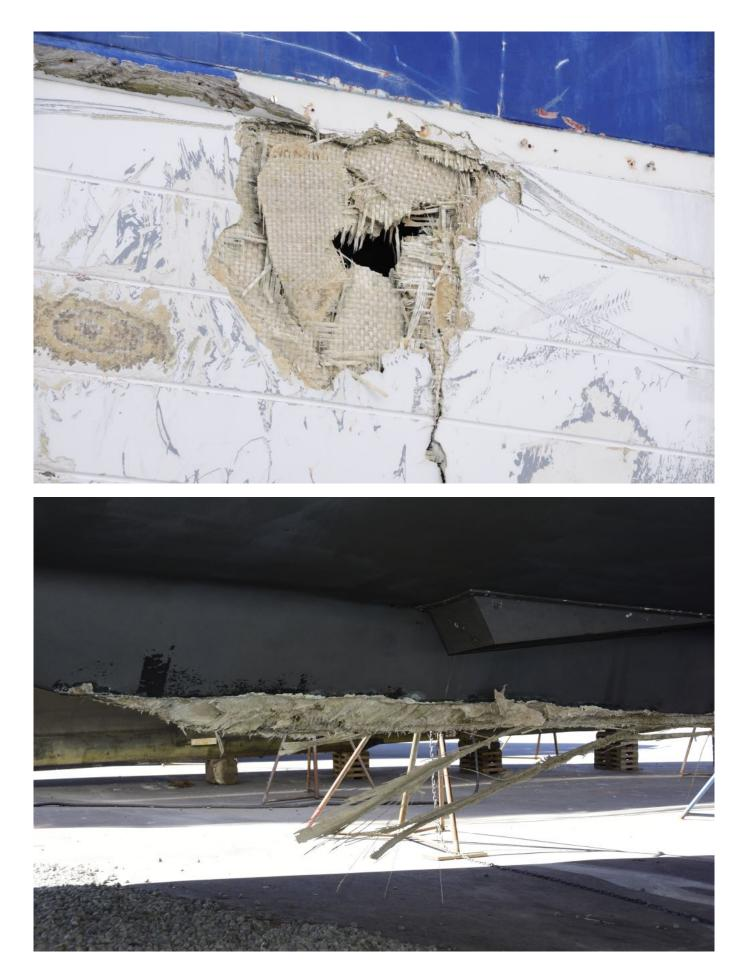
Collision and grounding damage, this will require secondary
