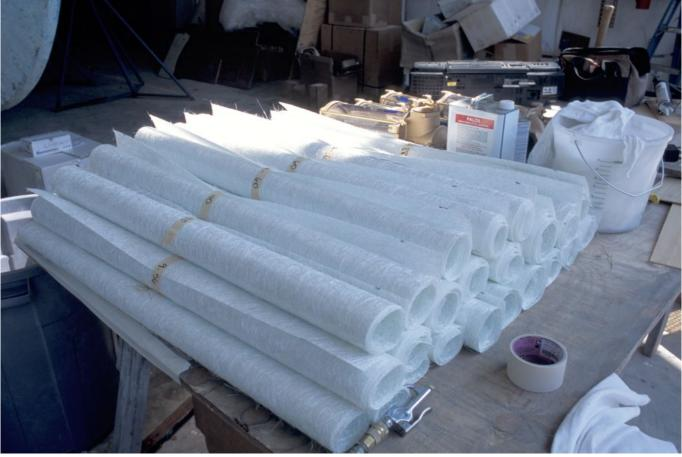
Fiberglass is a simple combination of fabric and resin, each successive layer adding strength and stiffness. Primary bonds are achieved when the resin is not fully cured, with secondary bonds coming into play after the substrate is no longer "green".
