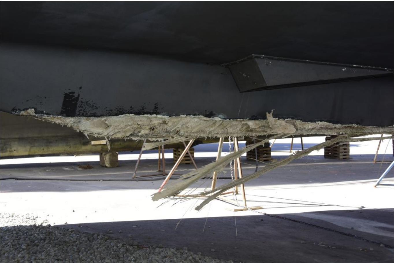
Collision and grounding damage, this will require secondary
