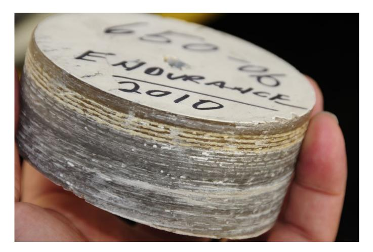
Each laminate is a separate layer of fabric and resin, which looks somewhat like tree rings when section cut. The one shown here includes four layers of Kevlar.
