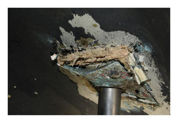
For highly loaded parts like this grounding-damaged strut, the importance of achieving a strong, reliable secondary bond cannot be over-emphasized.
