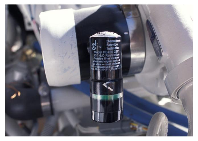
A stock air filter telltale vacuum indicator. Not really a gauge per se, more of an "idiot light", it will show red when the filter is restricted.
