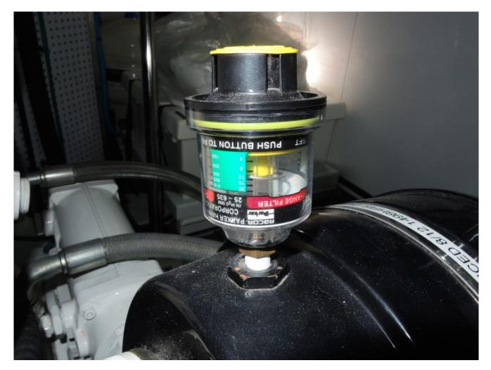
This air filter vacuum indicator gauge is clearly graduated, allowing the user to monitor progressive restriction, and providing ample warning for replacement.
