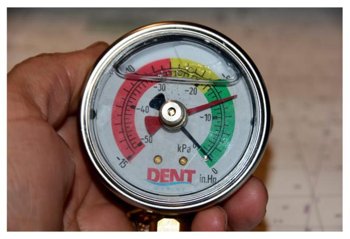
With its liquid-filled case to resist vibration, and a larger scale (representing a smaller and thus more accurate range), this fuel filter vacuum gauge represents the state of the art.
