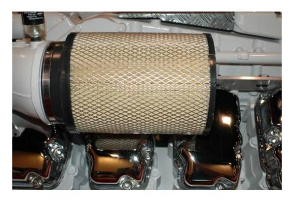
Air filters for modern diesel engines are costly; most are replaced needlessly, based on annual service guidelines rather than air flow restriction.
