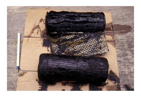
Engines will often continue to run even when filters are extremely contaminated, as are the ones shown in this image. This engine ran, however, at what price, was contamination making its way to the injection system? A vacuum gauge would have alerted the user to the need for filter replacement long before they became this impacted.
