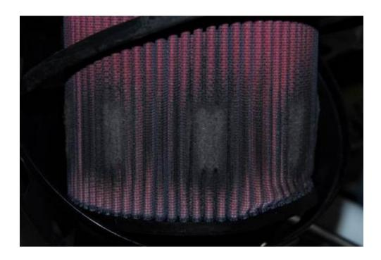
When viewed through air intake ports that surrounded this air filter, debris appeared to be severe. However, it's localized (it should, however, be addressed as it may be an indication of disintegrating engine room insulation) and had little effect on the restriction gauge.
