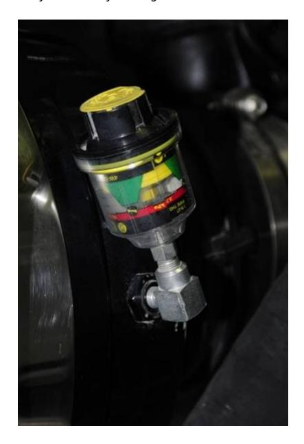
Air filter restriction gauges like the one shown here alert the user to the need for replacement.
