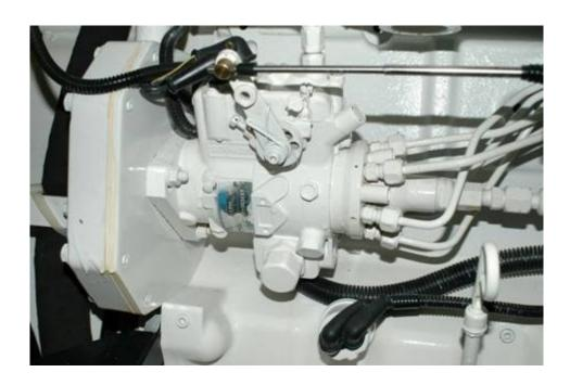
Fuel injection pumps may suffer cavitation damage when starved for fuel, a scenario that can occur when engines are operated with clogged fuel filters.
