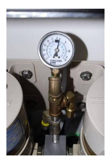
A stock fuel filter vacuum gauge; this one lacks a drag needle, making it necessary for the operator to monitor it while under way to determine the amount of restriction.
