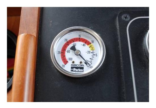
An in-dash fuel filter vacuum gauge enables the operator to monitor, in real time, fuel restriction for any reason, be it a clogged filter or some other fuel supply issue.
