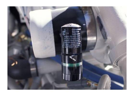
Most air filter restriction gauges show some sort of color coded indicator, green for all clear, for instance, and red for excessive restriction.
