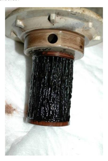
Engines may continue to operate with seeming normalcy even when filters are severely clogged. The insidious side effects, however, can include premature failure of diaphragm-type lift pumps.
