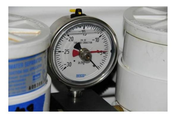
A more advanced vacuum gauge, it is liquid filled and therefore vibration dampened. The drag needle records the highest reading and retains it for viewing at any time, even when the engine is off.
