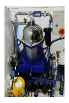
The mother of all polishing systems, centrifuges are capable of slinging water and dirt out of fuel down to a single micron, and they do so using centrifugal force rather than filter elements.
