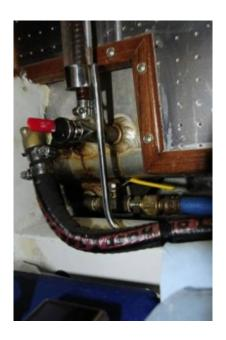
Polishing system pick up fittings should be located at the absolutely bottom of a fuel tank. While appropriate for supplying fuel to an engine, fittings like the one shown here are not low enough for polishing system use.
