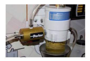
At the other end of the spectrum from high volume pumps, this prototype Lilliputian supplemental filtration system works by filtering fuel at a very low volume, albeit continuously.
