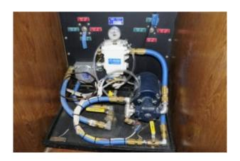
Most high volume polishing systems rely on either geared, like the one shown here, or multi-chamber diaphragm pumps. The plumbing used must be of sufficient diameter to accommodate the flow rate of these pumps.
