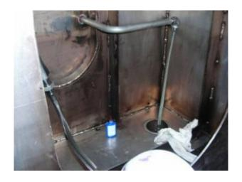
In order to work effectively, polishing system pickup and return plumbing must be plumbed to opposite ends, and always
