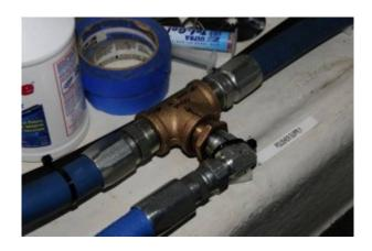
Like fuel plumbing for the engine, polishing system plumbing must be robust, leak-proof and flame resistant.
