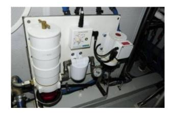
High capacity polishing systems like the one shown here, are often palletized, they include filter, high volume pump, and a control mechanism or timer, along with a vacuum gauge.
