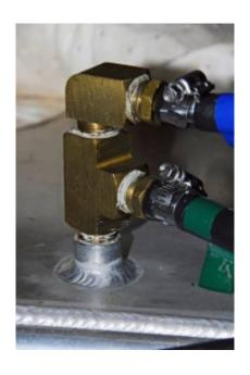
A textbook example of paralleling, sharing fuel pick up and return fittings with the vessel's main engine. This approach severely restricts a polishing system's capabilities, as well as potentially starving an engine of fuel, and should therefore be avoided.
