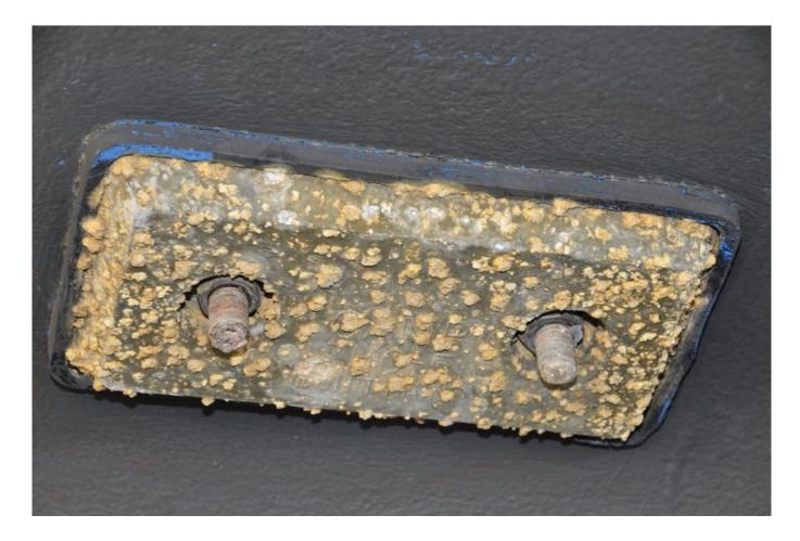
When exposed to fresh water, zinc anodes develop a coating that effectively renders them inert. It can be scrubbed off using a non-metallic brush or pad, however, until this is done, or they are replaced, the vessel's corrosion protection level remains diminished.
