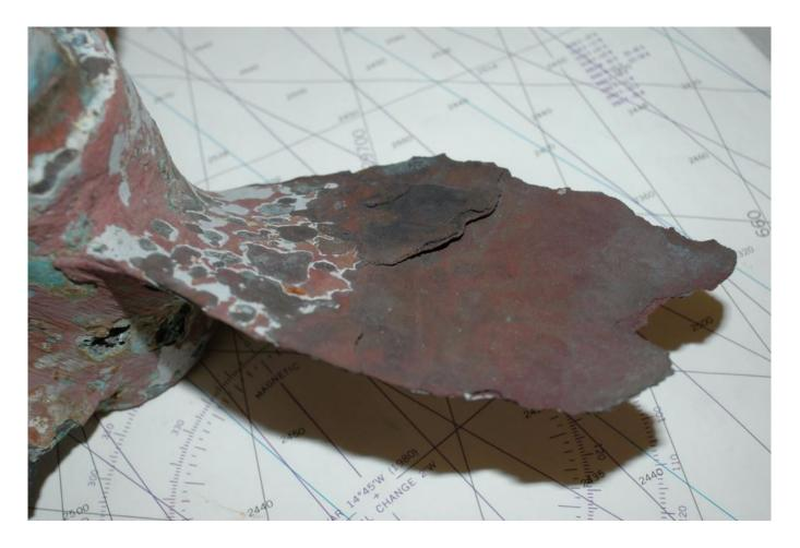
Stray current corrosion, which is nearly always the result of DC current leaking into and around the water in which a vessel floats, via faulty wiring, is both rapid and highly destructive. It can lead to damage like the that shown here over the course of days or even hours.
