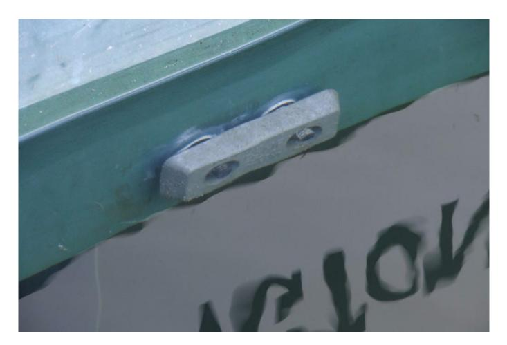
Unlike zinc, aluminum anodes are designed to operate effectively in salt, brackish and fresh water with little or no degradation in performance.
