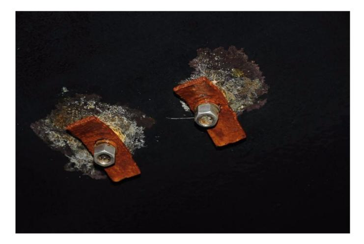
Monitoring and replacing anodes in a timely fashion is a critical aspect of a corrosion prevention plan. Waiting until they completely disappear, like the one shown here, only its armature remains, on the other hand, makes galvanic corrosion a near certainty. The smaller an anode becomes, the less protection it offers.
