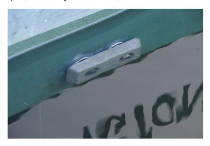
Unlike zinc, aluminum anodes are designed to operate effectively in salt, brackish and fresh water with little or no degradation in performance.
