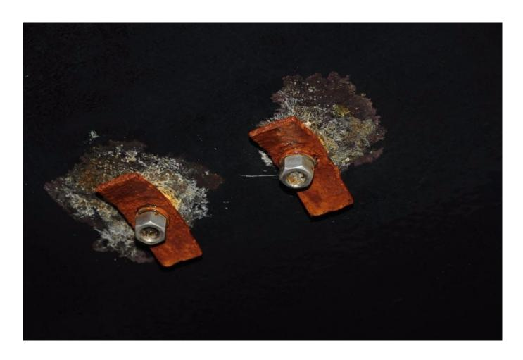
Monitoring and replacing anodes in a timely fashion is a critical aspect of a corrosion prevention plan. Waiting until they completely disappear, like the one shown here, only its armature remains, on the other hand, makes galvanic corrosion a near certainty. The smaller an anode becomes, the less protection it offers.
