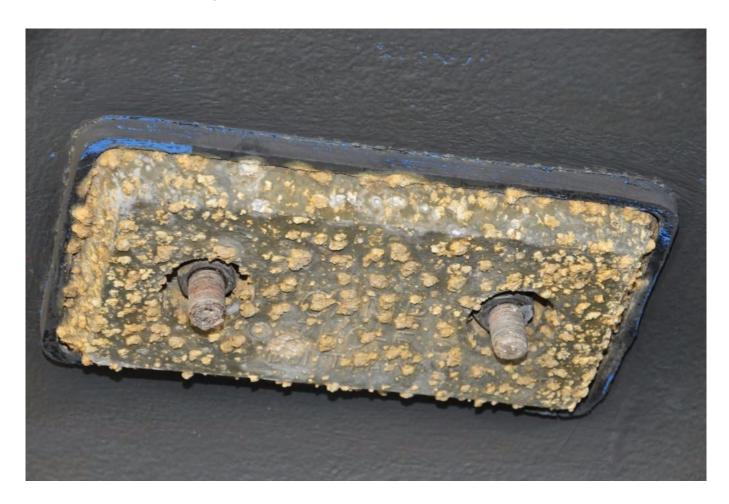
When exposed to fresh water, zinc anodes develop a coating that effectively renders them inert. It can be scrubbed off using a non-metallic brush or pad, however, until this is done, or they are replaced, the vessel's corrosion protection level remains diminished.
