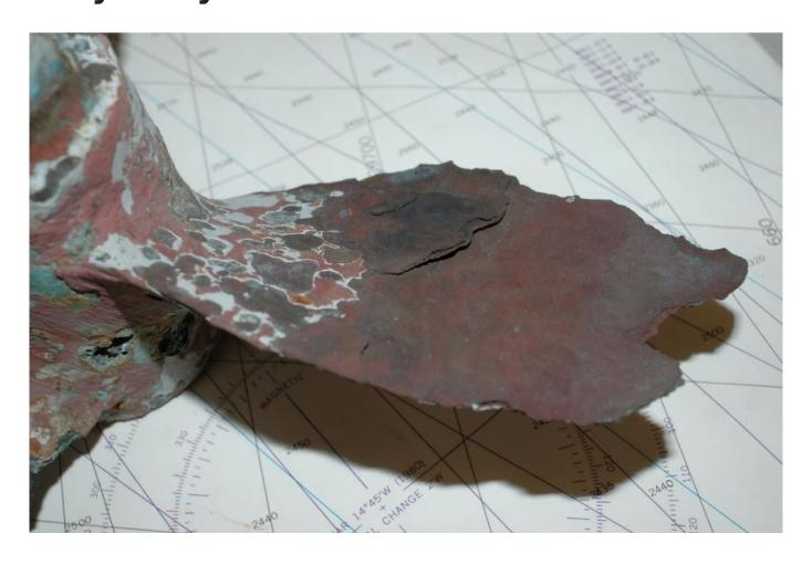
Stray current corrosion, which is nearly always the result of DC current leaking into and around the water in which a vessel floats, via faulty wiring, is both rapid and highly destructive. It can lead to damage like the that shown here over the course of days or even hours.
