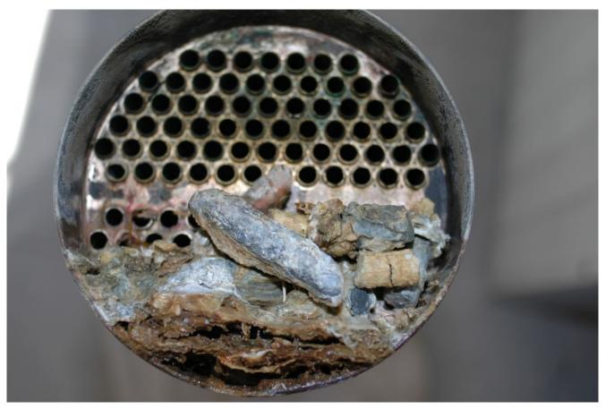
Depleted anodes are among the most common sources of heat exchanger performance issues. Heat exchangers should be accessed at least every two years for inspection and cleaning. It's the radiator of your marine engine, however, unlike an automobile, your marine engine transfers its waste heat, via its closed cooling system, from coolant to seawater rather than air, using a heat exchanger.
