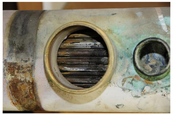
The coolant side of a heat exchanger, while not as prone to clogging as the raw water side, should be periodically inspected. If the engine has experienced an overheat, the closed cooling side should be cleaned/descaled, as overheated coolant can leave an insulating film on the tube bundle, which will decrease heat transfer.
