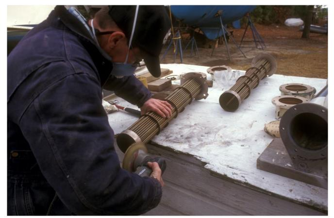
For larger heat exchangers, tube bundles are removable for cleaning, and repair. Here a technician removes scale using a ScotchBrite disc.
