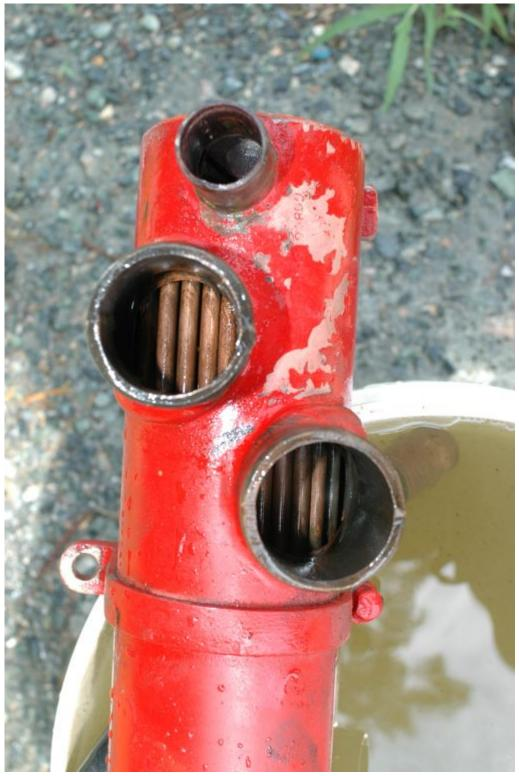
Scale build up can slowly diminish heat transfer within a heat exchanger. Often, this manifests itself when the engine is run harder than usual. All properly maintained diesel engines should be capable of running at high load, approximately 75%, indefinitely, and full throttle for 5-10 minutes, without overheating.
