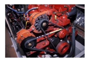
Horsepower is often measured without an engine's belt and gear driven accessories such as pumps and alternators. Depending on their size, and the size of the engine, these can have a noticeable change on ultimate power transmitted to the propeller.
