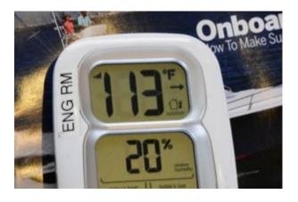
Excessive engine room temperature, and specifically the temperature of the air the engine is ingesting, can have a significant impact on horsepower production.
