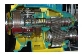
As is often the case, there's no free lunch when it comes to gears. A reduction gear, the stacked beveled gear set on the right in this demonstration cut-away transmission, offers increased torque while reducing rpm. The price paid is added friction and a resultant slight loss in efficiency.
