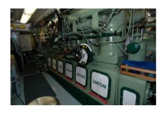
Very large, slow-turning diesel engines like the one shown here, aboard the MV Union Jack, are capable of producing mountains of torque at relatively low horsepower.
