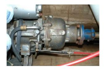
Reduction gears are tantamount to adding a cheater bar to a socket wrench, enabling a high speed engine's rpm to be converted to additional torque. In this example, the reduction gear is the bell-shaped device, on the right, bolted to the output side of this transmission.
