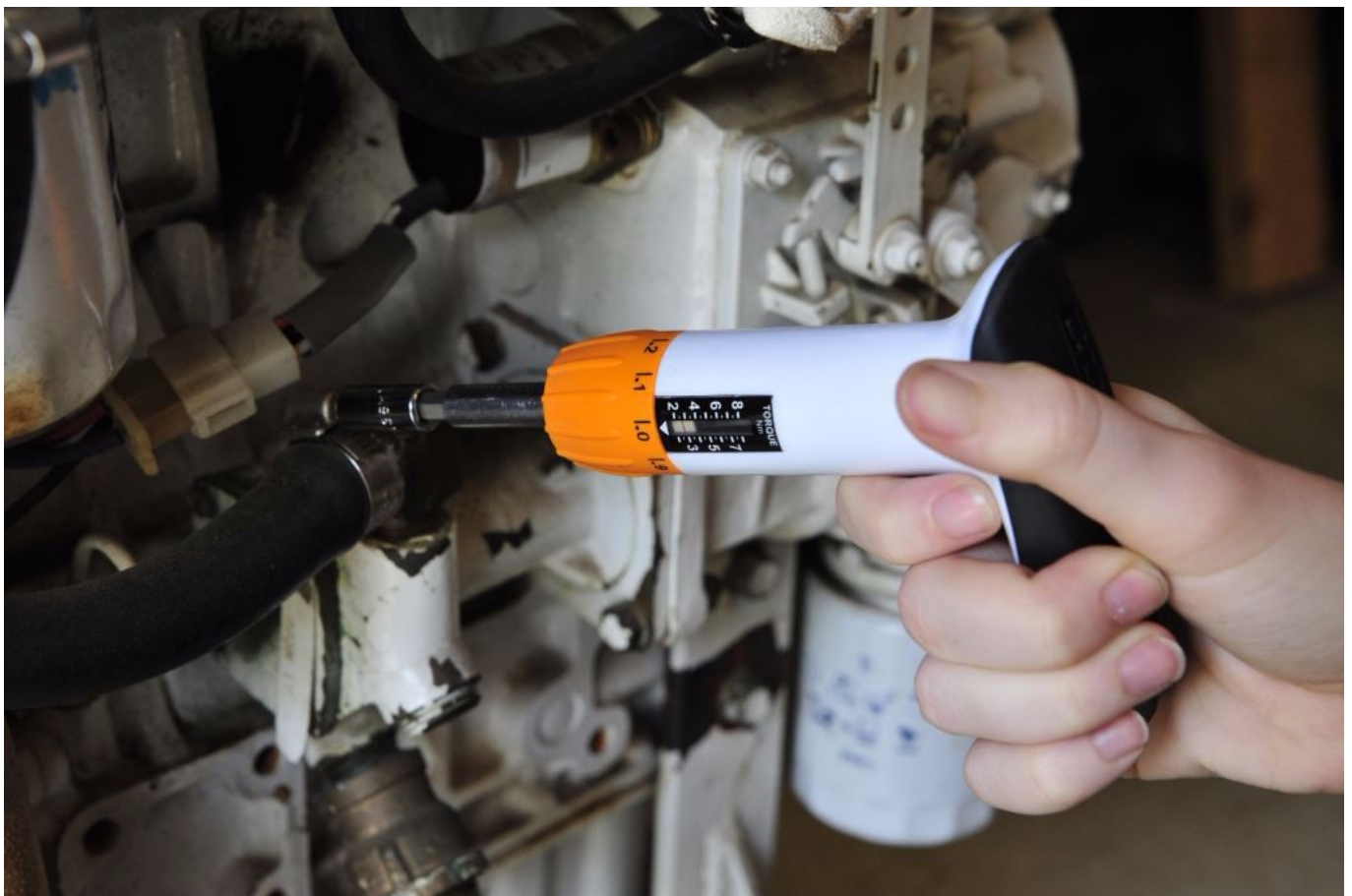
A mini-torque wrench being used to ensure proper hose clamp tension.
