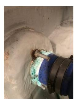
The green ground wire to this part is clean and securely attached to one of the 3 bolts holding the part in place in the shaft log. Zincs on the prop shaft, trim tabs and main zinc on the transom (to which all green wires terminate) are doing their job and are replaced each year. The raw water strainer for engine cooling and the smaller strainer for the A/C have a similar greenish tinge to the surface but no fuzzy material that can be removed. Both strainers have green grounding wires.
