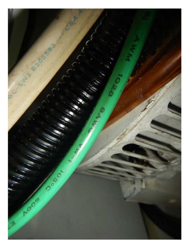
The vast majority of onboard AC power circuits include at least three wires, a "hot", sometimes referred to as "ungrounded", which is usually black or red, a "neutral", or "grounded" wire, which is white, and a safety ground, which green, and is more accurately referred to as a "grounding wire" because it normally carries no current, unless it is
