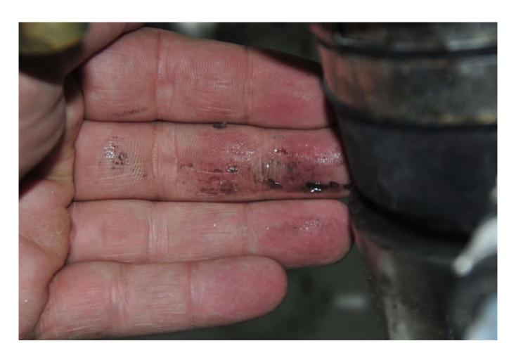
Dripless shaft seals should be dripless, they should not leak. In some cases they may leak slightly and initially until broken in, however, this should not last more than a few hours. If it does, something is wrong.
