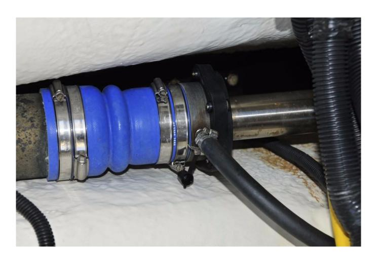
Most dripless stuffing boxes rely on a ultra-flexible hose to allow the sealing portion of the assembly to align to and "float" on the shaft. If the shaft is not centered in the shaft log, or if the shaft vibrates excessively, leakage can result.
