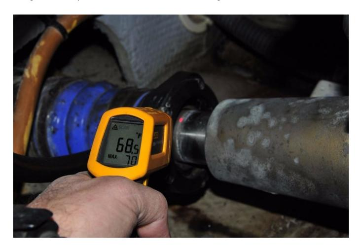
Temperature remains a valuable indicator of a seal's functionality, if it's significantly hotter than the water in which the vessel floats, it's almost certainly not receiving enough flow. If they get hot enough both lip and face seals will overheat, and fail, which will lead to leaking.
