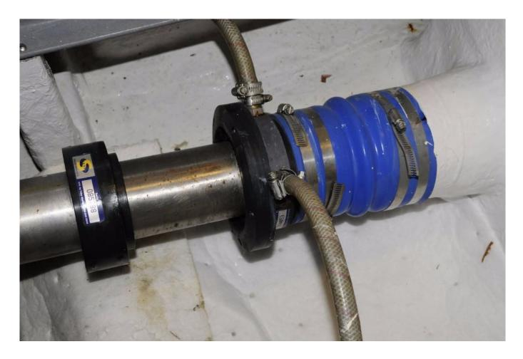
The hose used to supply water to the stuffing box must be flexible, however, PVC hose such as that used for potable water, shown here, should not be employed, as it lacks the necessary robustness for raw water use.
