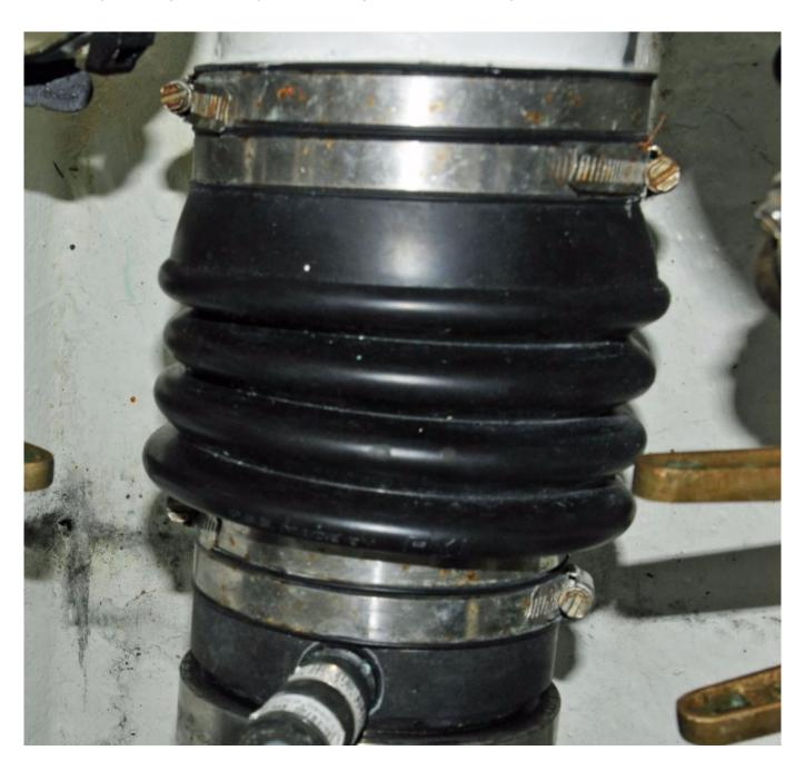
This bellows is over-compressed, so much so that it is over-riding its hose clamps, visible at the bottom of the image.
