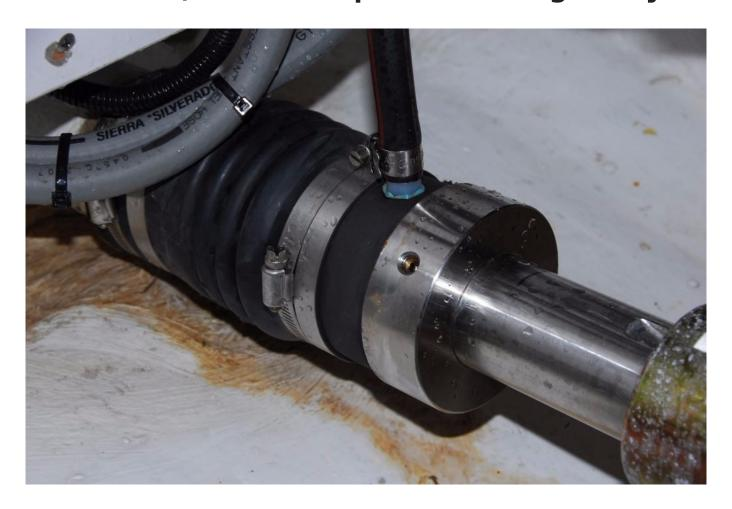
Face seals rely on the spring tension created by a bellowstype hose. The system is simple and effective.
