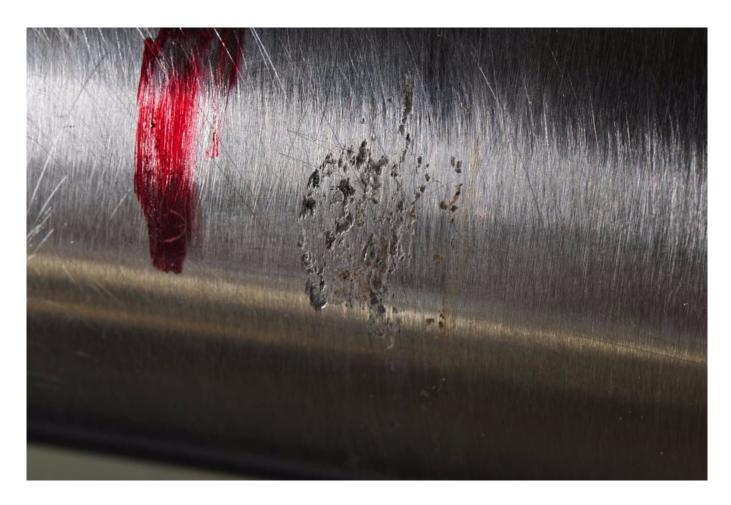
Prop shafts must be free of pitting or other irregularities where face seal 0 rings and especially lip seals reside, the latter are more sensitive to this issue. If the surface is not smooth, it will be difficult to achieve a watertight seal.
