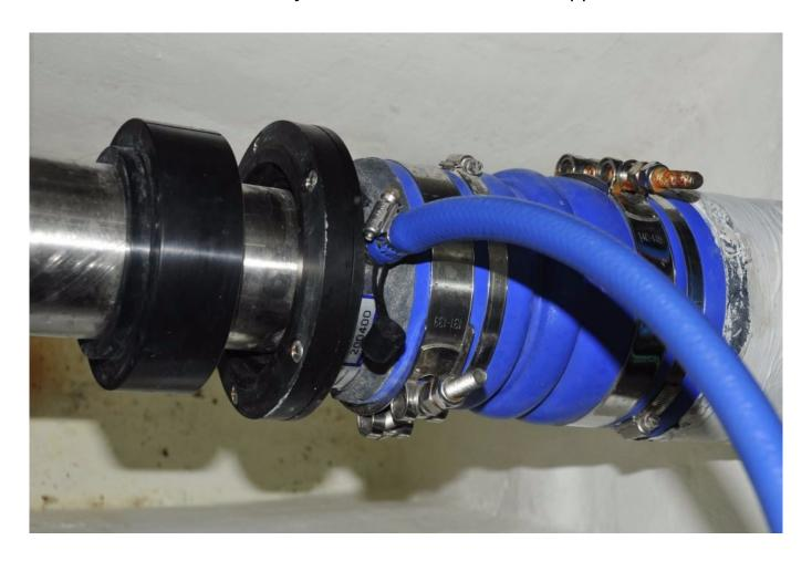
Lip seals like the one shown here are self-centering, they rely on the interface between the lip and the spinning shaft to make a watertight seal. The one shown here is equipped with a spare seal carrier, which retains and protects a set of replacement seals.
