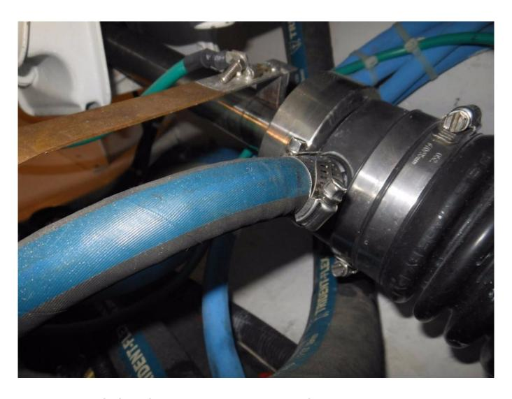
The water injection hose must be flexible enough to allow the a dripless stuffing box to float, if it's too rigid, or too short, it can side load the seal, causing it to leak.
