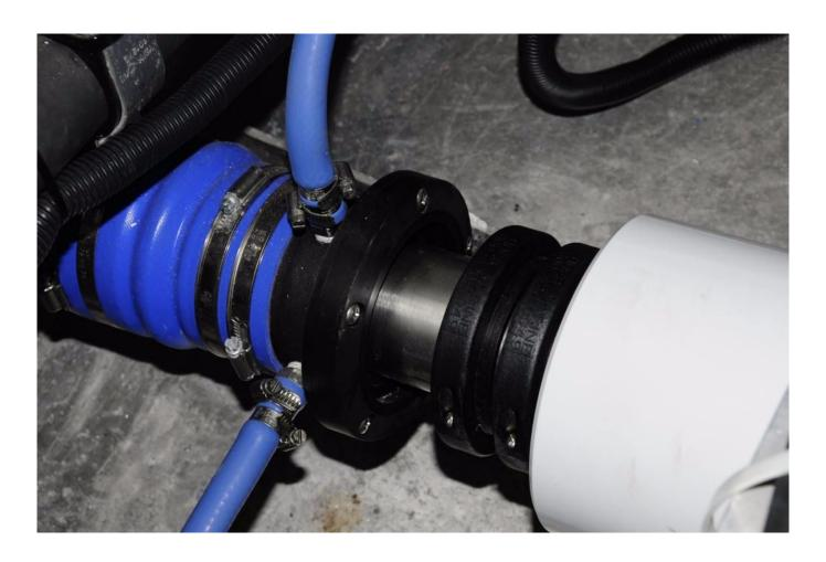
Fort twin screw applications, dual water injection enables one engine to supply water to both seals when operating on one engine. The stuffing box shown here includes an optional second injection point, which is paralleled with the other shaft's stuffing box.
