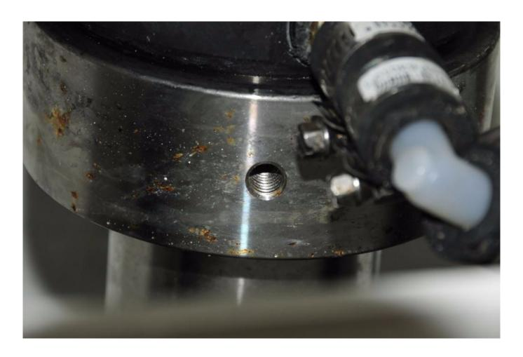
Face seals rely on stacked set screws to secure the rotor. In many cases the second set screw is, like the one shown here, not installed.
