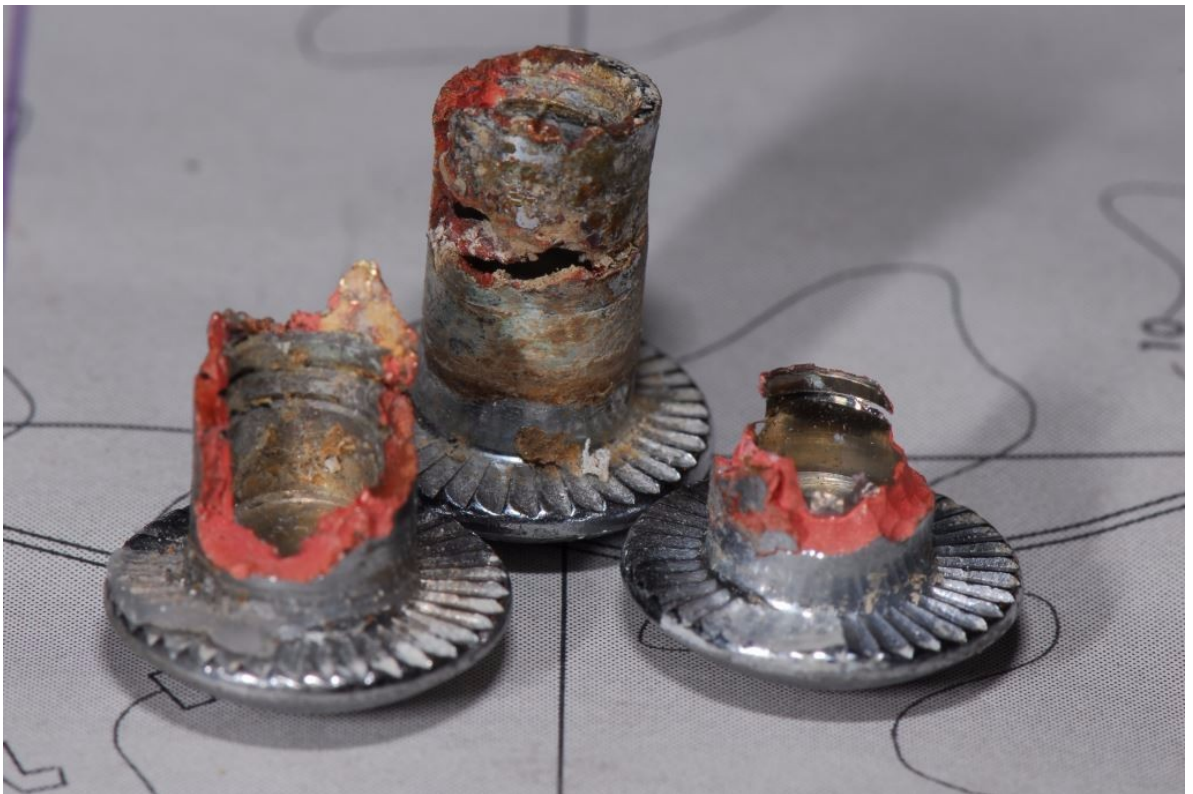
These chrome-plated brass sex-bolts, installed in a
