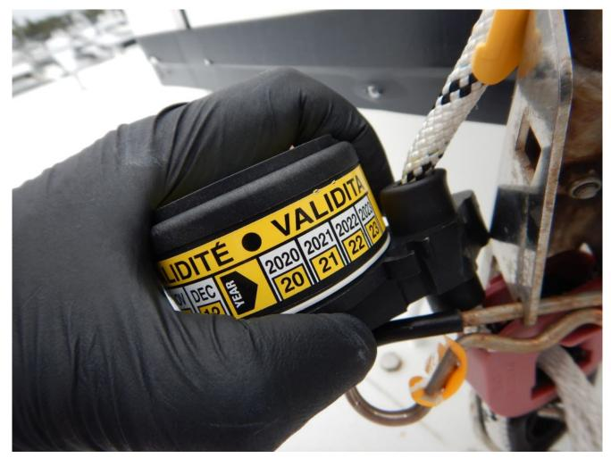
HRU's must have their expiration date, two years from the date of installation, permanently scratched into the unit's decal. Marking with a felt-tip pen is not acceptable.
