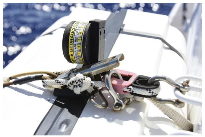
Hydrostatic and manual release units located side by side. The painter can also be seen, shackled to the weak link device.
