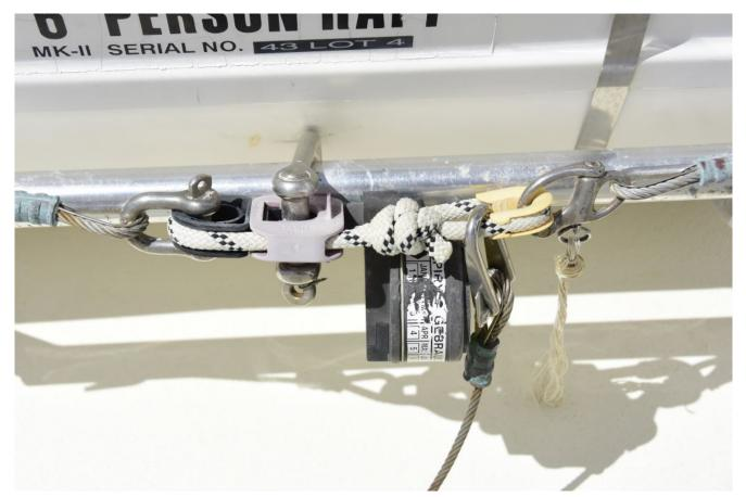
The number of ways a HRU can be installed incorrectly is seemingly endless. This HRU has been shackled to the cradle using its weak link port.
