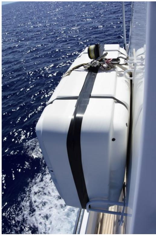
Vertically-mounted rafts are more prone to water entry via the seam between the canister halves. The tape that covers, or gasket that fills, this gap should be inspected regularly.
