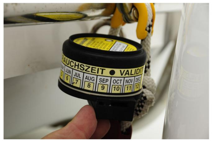
A HRU that is in service, and has no indicated expiration date, should be removed, discarded and replaced with a new unit that is dated as soon as it is installed A Tale of Two Straps
