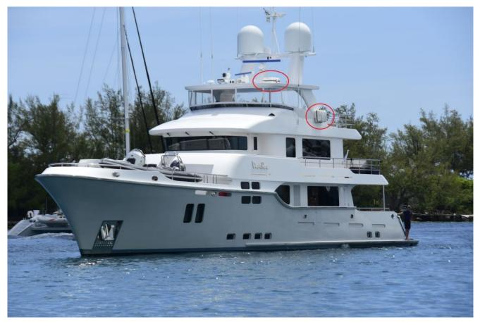
This vessel has four 8 person rafts, two located on the sides of the flybridge hard top supports, and two on the hardtop. These locations provide a good mix of access and protection.
