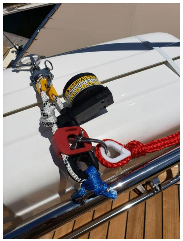
While this painter is properly secured to the HRU weak link, the small ring on the manual release snap shackle lacks a lanyard. Under load, this will be difficult to release. The blue lashing would be better served by a shackle.
