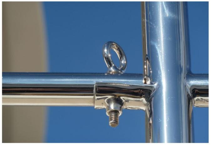
A removable rail section on a Fleming 55, facilitating easier life raft deployment.
