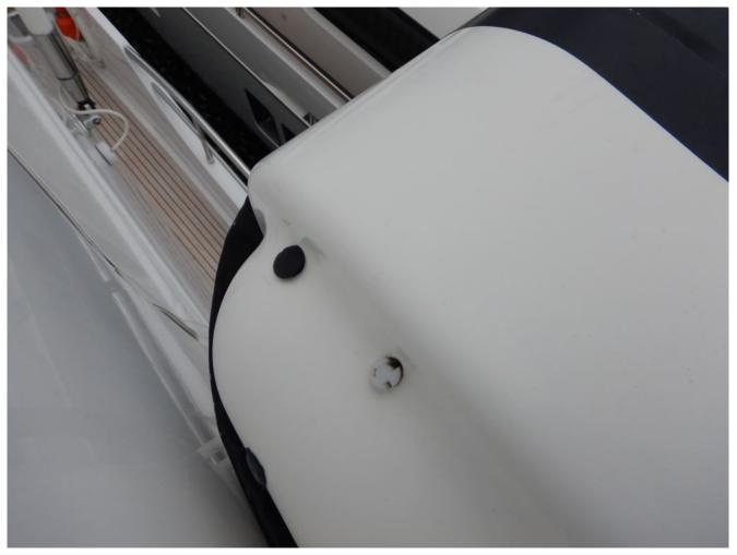
This vertically-installed raft's upward-facing drain is an invitation to water entry. When rafts are purchased, or serviced, the dealer or servicing agent should be made aware of the intended installation orientation, so he or she can cap the upper holes.
