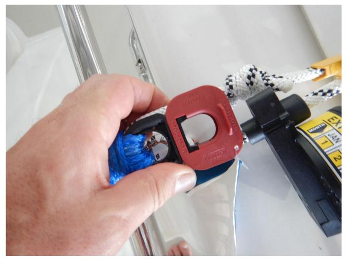
This weak link attachment point has not been used, instead this raft's painter has been incorrectly attached elsewhere, which means it does not have the benefit of automatic release as the vessel sinks.
