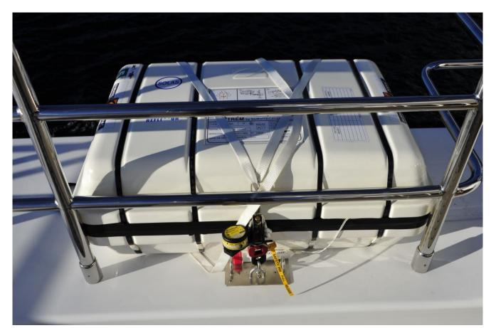
Excess strap material should be trimmed or neatly bound and secured so as not to hinder the hydrostatic deployment of a raft.
