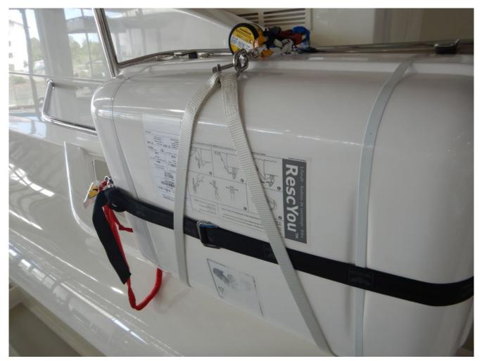
This raft has been inadvertently equipped with both manual (black) and hydrostatic (white) lashings. If the vessel were to sink, the raft would be unable to float free even after the HRU was triggered.
