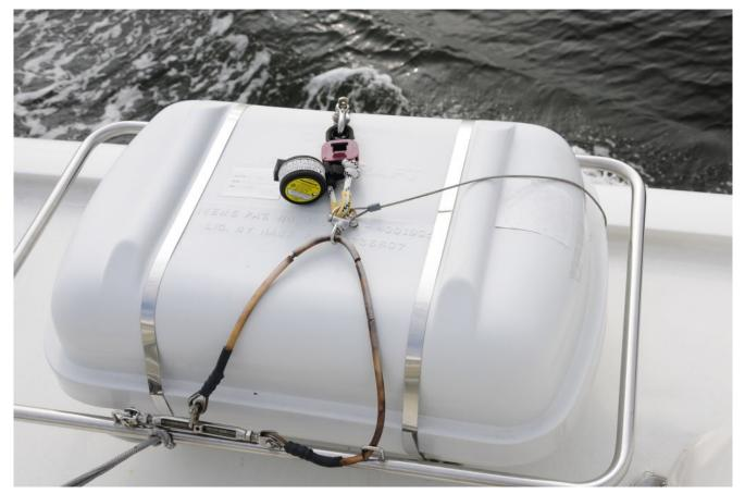
If this raft is deployed manually, the painter will be released, and the raft will not inflate.
