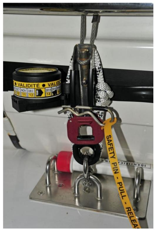
While this raft's painter is not attached in the proper location, the means of manual deployment is clearly identified.
