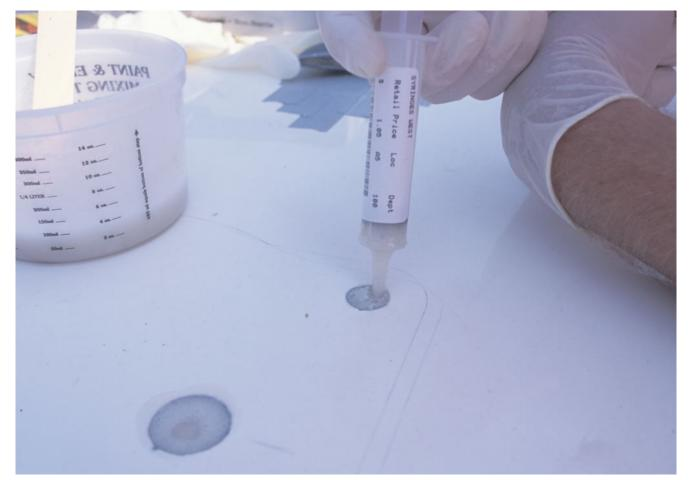
When installing cradles on fiberglass cored composite structures, such as decks and cabin tops, it is imperative that the core be removed and back filled with epoxy at each fastener penetration.
