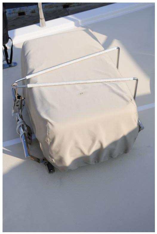
Canvas covers can extend the life of a raft canister and gaskets, and reduce the likelihood of water leaks, however, they must be removed when the vessel gets underway.
