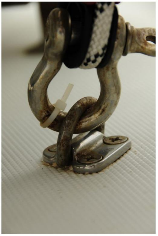
Hard points for raft and painter attachment must be sturdy, they must rely on through bolts rather than tapping screws, and they must remain corrosion-free.
