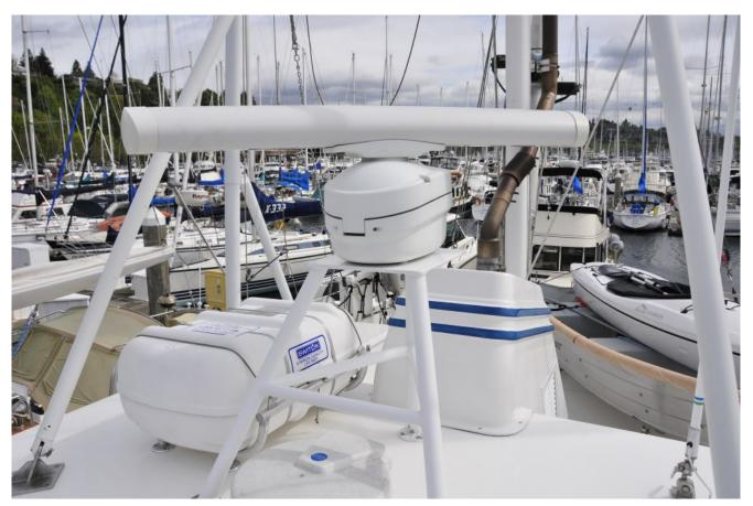
There are times where a compromise must be struck. A high location, away from green water and out of high traffic areas is ideal, however, the rigging and gear above and around this raft could prove an entanglement hazard.
