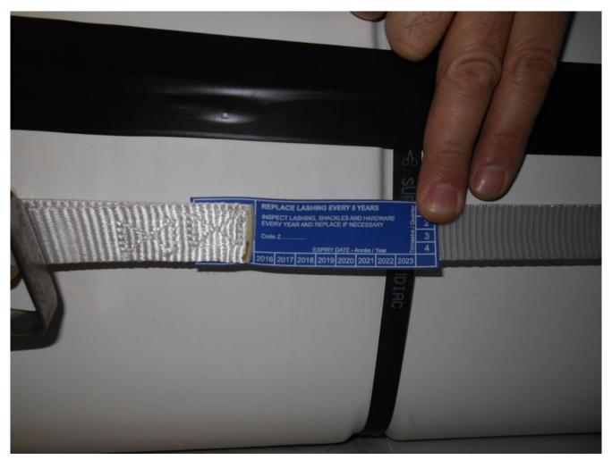
Vertically-mounted rafts do not have the benefit of gravity for support. Their lashings, and the lashings of all rafts, must be inspected regularly and replaced at the first sign of deterioration, or when they have reached their expiration date.
