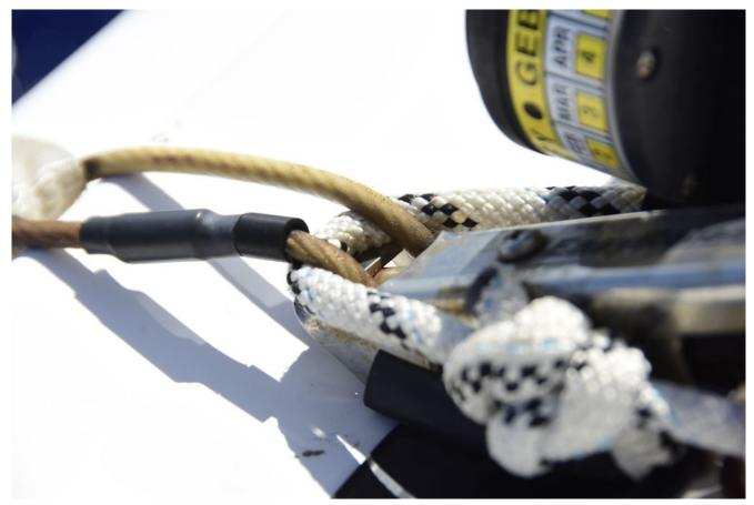
While manual release units do not have an expiration date, they should be routinely inspected for deterioration.
