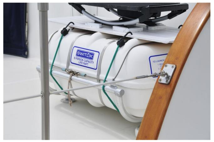
For manual and hydrostatically released rafts, nothing should hinder their deployment. Keep all gear and equipment off of and away from raft canisters.
