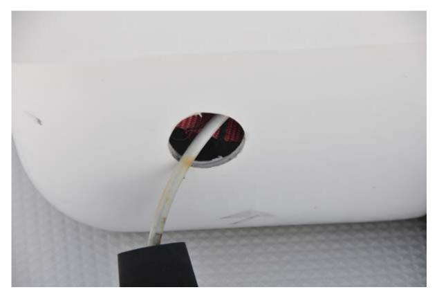
Water entry into raft canisters is an ever present danger. Rafts cannot be inspected too frequently for potential water entry points.
