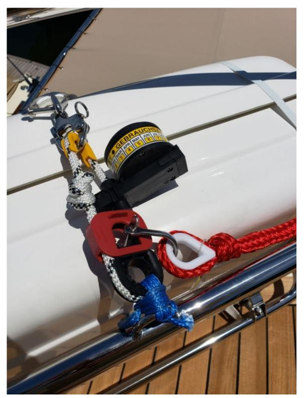
While this painter is properly secured to the HRU weak link, the small ring on the manual release snap shackle lacks a lanyard. Under load, this will be difficult to release. The blue lashing would be better served by a shackle.
