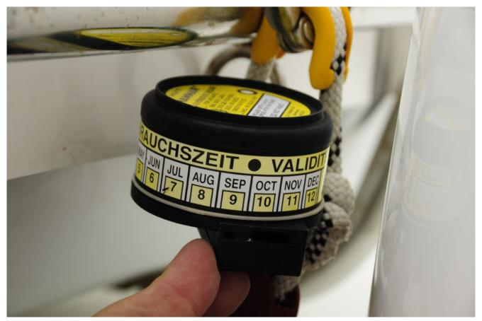
A HRU that is in service, and has no indicated expiration date, should be removed, discarded and replaced with a new unit that is dated as soon as it is installed
