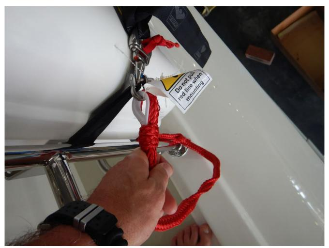
This painter line has been attached to the manual release lashing (pulling on the red toggle will open the hook). For rafts that are not equipped with a HRU, and 'weak link' painter attachment point, the painter should be securely attached to the raft cradle or a stout pad eye.
