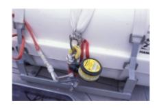
The familiar hydrostatic release mechanism. Like flares, EPIRB batteries and life rafts themselves, these require inspection and periodic replacement. Also, counterfeit units have been encountered, so make sure yours is genuine by contacting the manufacturer for verifying features or serial numbers.
