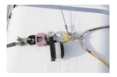
Make certain you understand how life raft security and deployment mechanisms are designed to work, don't assume they've been properly rigged. In the manner in which this raft's release mechanism has been installed, if it were to deploy manually the raft would <u>not</u> inflate nor would it remain attaced to the vessel.
