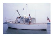
The hydrostatic release equipped raft aboard this vessel deployed when she was swept by a moderately (when compared to the size of the vessel) sized wave. The empty raft cradle can be seen to the right of the crew member standing aft.
