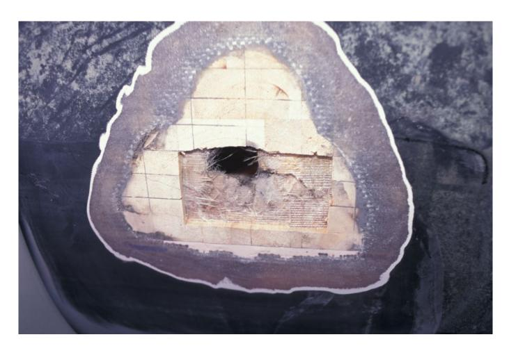
This vessel suffered structural hull damage at the waterline, the result of a lightning strike.
