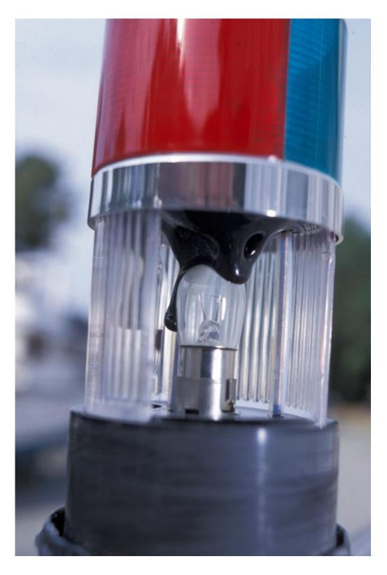
A mast head tricolor light damaged by a lightning strike.
