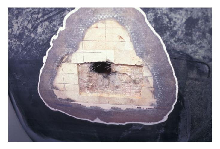
This vessel suffered structural hull damage at the waterline, the result of a lightning strike.
