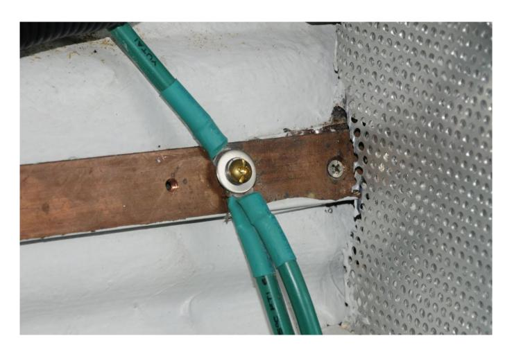
While not immune from damage, a well-bonded vessel is more resistant to the effects of a nearby or direct strike.
