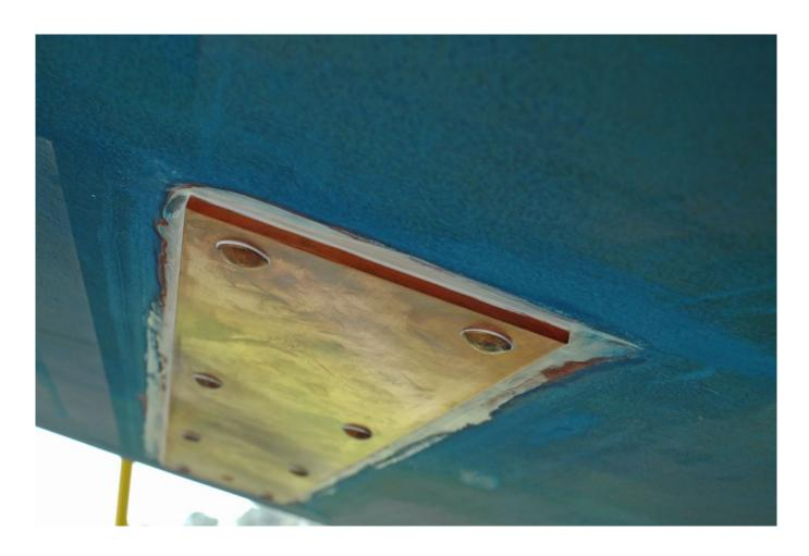
Because the edges do the dissipating, the longer the ground plate the better.
