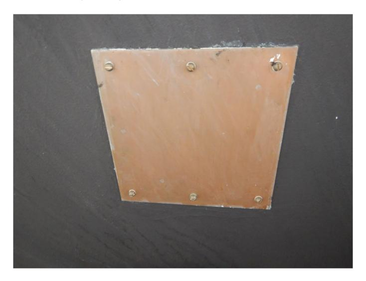
ABYC Standards call for a minimum of one square foot of metal plate to be used as the ground terminal.
