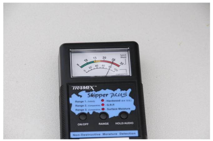
Most moisture meters utilize different scales, in this case for fiberglass (GRP), timber and surface moisture. It's
