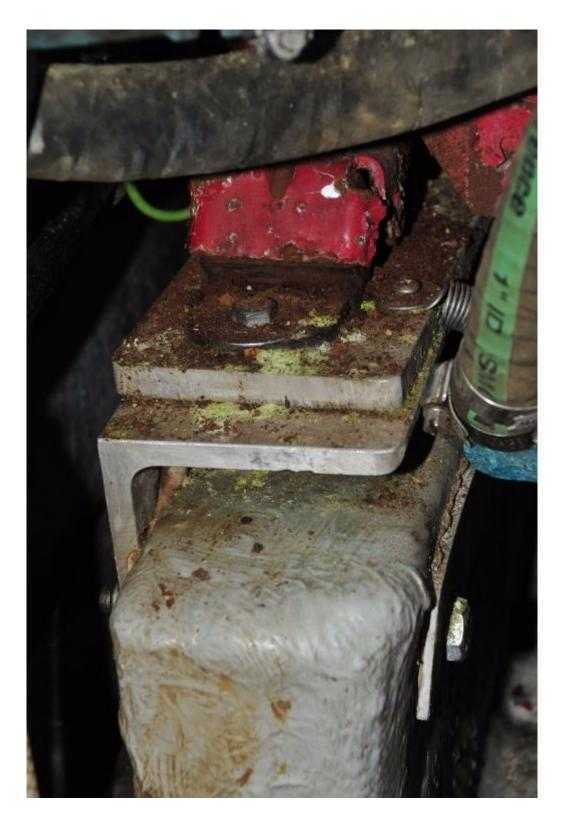
Even with the best of intentions, there are many ways a motor mount installation can go wrong. In this case the most egregious is the cantilevered "diving board" support bracket. Not only is this prone to failure, it's also likely to compound vibration.
