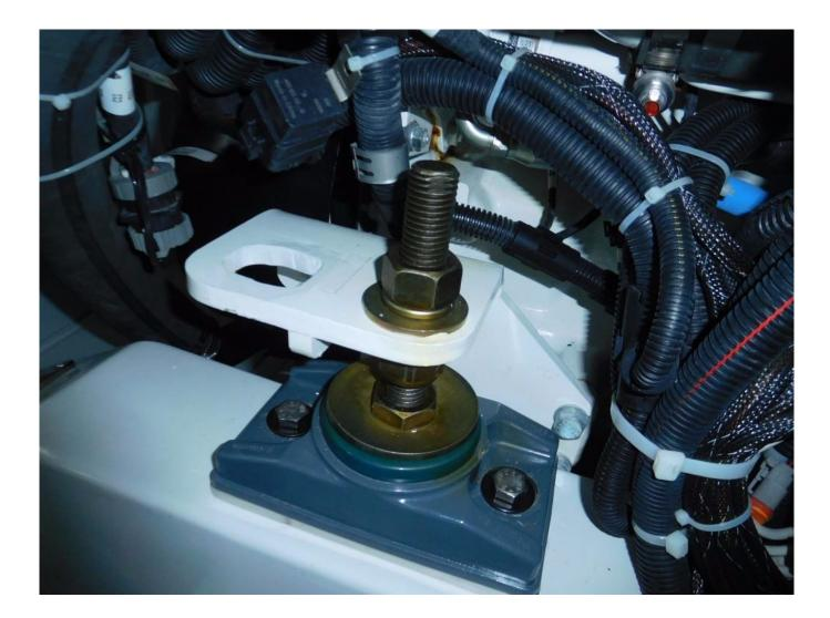
Corrosion is an ever present issue where motor mounts are concerned. The base of this mount is made from composite, it will therefore never rust. The adjustment stud has been coated with a film corrosion inhibitor that dries to a waxlike consistency. Note the aluminum shim beneath this mount.
