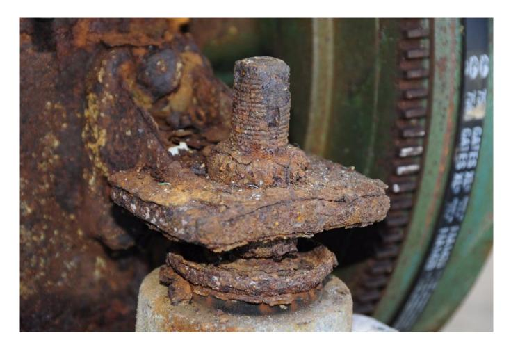
Motor mounts are adjustable and while they may not need to be adjusted often, they must be kept free of corrosion and in good working order.
