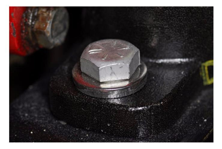
Standard, thin fender washers (top) and stainless steel bolts simply lack the necessary rigidity and tensile strength for use in many motor mount applications. The heavy duty thick washer (above), and grade 8 bolt, shown here provide the necessary support for the anticipated loads.
