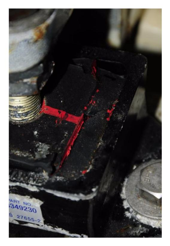
This motor mount utilizes a telltale red core to signal that it's reached the end of its life. In many cases a failure of this sort is the result of an installation error.
