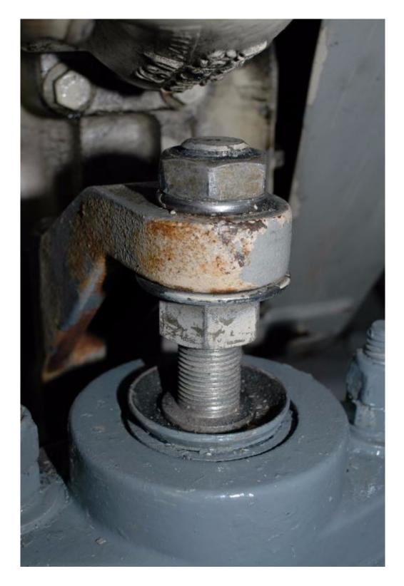
The engine's bracket or foot should reside somewhere in the middle of a motor mount's stud. This one is at the limit of its upward adjustment, exposing the mount to excessive load thanks to the added leverage.
