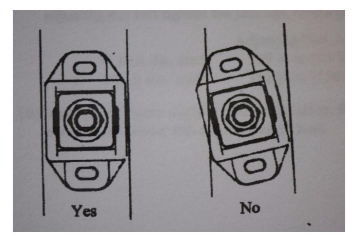
Avoid toe and camber when installing motor mounts, adjustment studs must be perpendicular with the engine bracket, and the mount base must be parallel with the crankshaft centerline and stringer or shim surface (diagrams courtesy Barry Controls).
