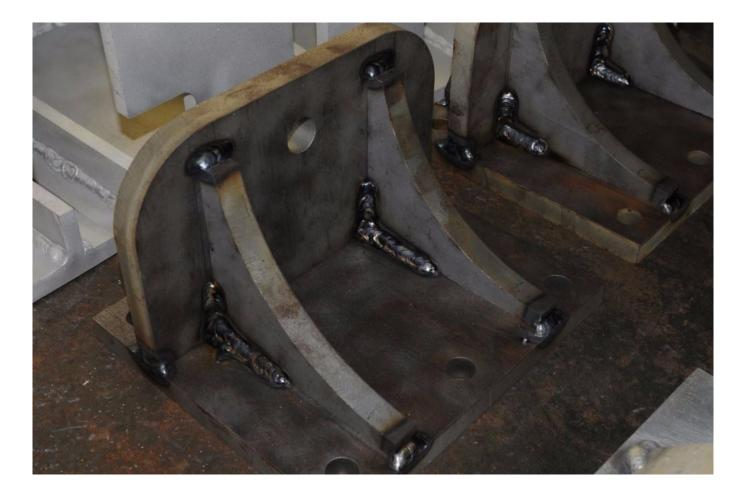
If a motor mount cannot be installed directly on a stringer, then a bracket must be fabricated. Brackets must be heavily built, and inflexible. The ones shown here are in the process of being fabricated to support a 790 hp engine.
