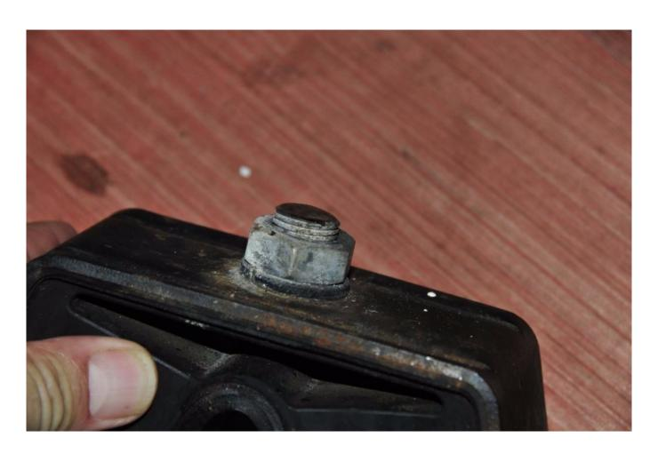
Over-extension (top) is a common issue with motor mount installations; often leading to failure of the stud (above). In spite of the composite shim that has been added to this mount, the problem remains.
