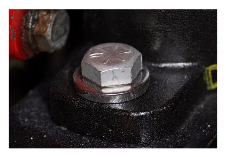
Standard, thin fender washers (top) and stainless steel bolts simply lack the necessary rigidity and tensile strength for use in many motor mount applications. The heavy duty thick washer (above), and grade 8 bolt, shown here provide the necessary support for the anticipated loads.
