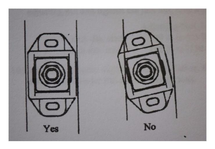
Avoid toe and camber when installing motor mounts, adjustment studs must be perpendicular with the engine bracket, and the mount base must be parallel with the crankshaft centerline and stringer or shim surface (diagrams courtesy Barry Controls).
