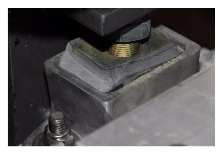
This mount is failing because it has been installed incorrectly, the surface on which it rests is not parallel to the engine's bracket in both planes, causing the rubber insert to deform.
