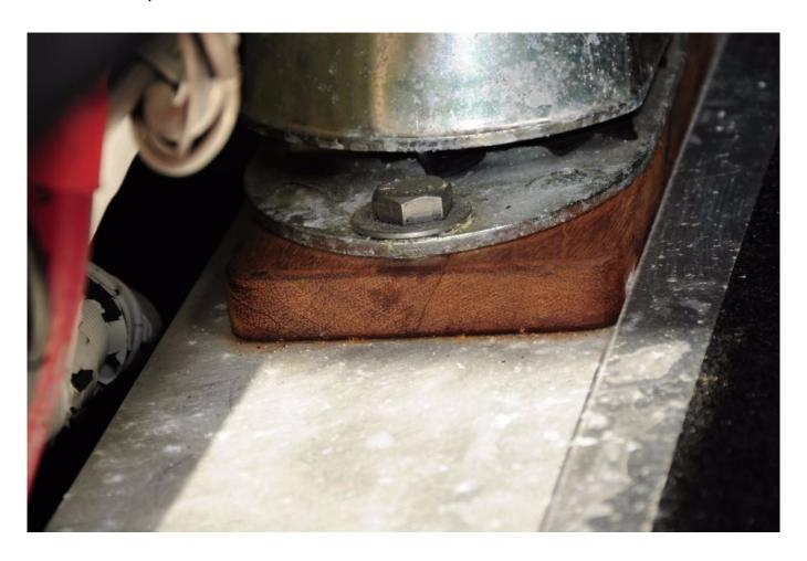
Because of its compressibility and propensity to crack, timber, even teak, is not a suitable material for shimming motor mounts.
