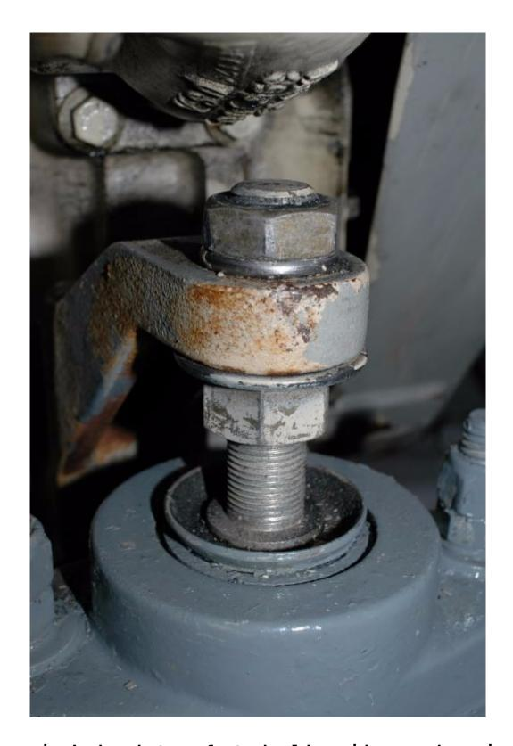
The engine's bracket or foot should reside somewhere in the middle of a motor mount's stud. This one is at the limit of its upward adjustment, exposing the mount to excessive load thanks to the added leverage.
