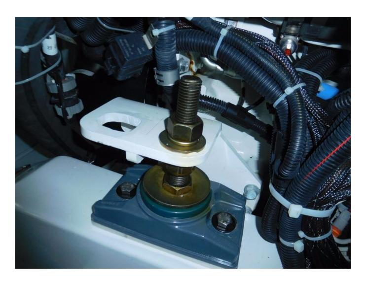
Corrosion is an ever present issue where motor mounts are concerned. The base of this mount is made from composite, it will therefore never rust. The adjustment stud has been coated with a film corrosion inhibitor that dries to a wax-like consistency. Note the aluminum shim beneath this mount.
