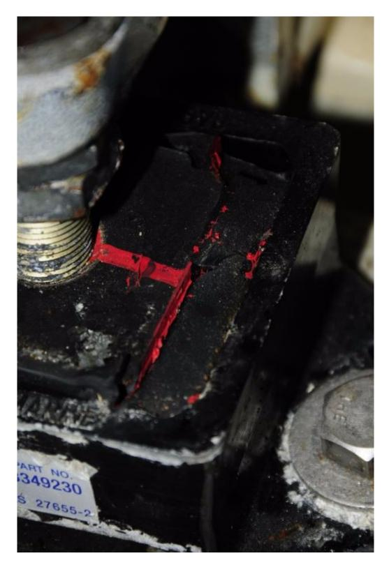
This motor mount utilizes a telltale red core to signal that it's reached the end of its life. In many cases a failure of this sort is the result of an installation error.
