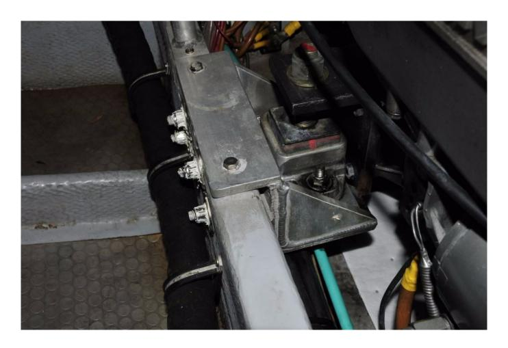
Motor mounts and their brackets should be gusseted, to prevent flexing, and through bolted.
