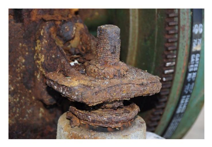
Motor mounts are adjustable and while they may not need to be adjusted often, they must be kept free of corrosion and in good working order.
