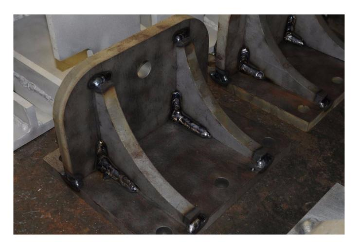
If a motor mount cannot be installed directly on a stringer, then a bracket must be fabricated. Brackets must be heavily built, and inflexible. The ones shown here are in the process of being fabricated to support a 790 hp engine.
