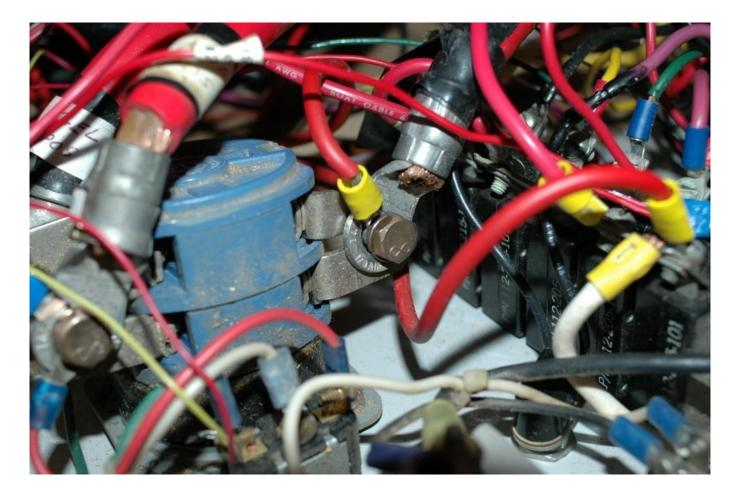
Wiring attention to detail plays a significant role in shore power safety. A small error, with no outward indication of a problem, can have life-threatening results.
