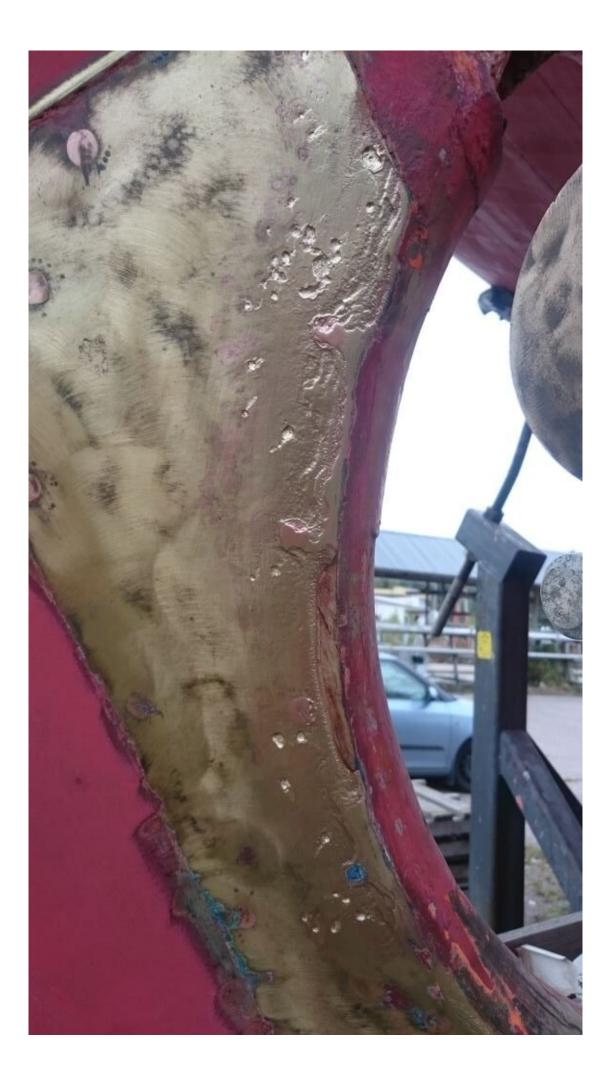
I had one zinc anode attached to the planking at stern with no electrical connection to any metal part (stupid!). It was almost as new.
