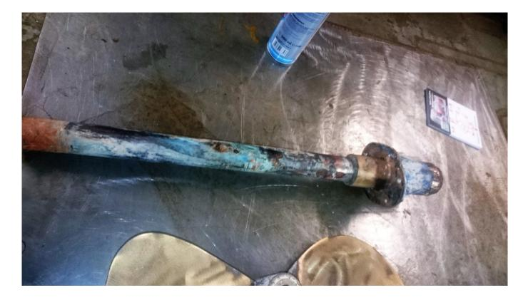
Severe damage had occurred at the 4-5 mm inch equivalent bronze plates that strengthen the rudder around the propeller opening. At the front edge closest to the propeller some 1 cm inch equivalent of the plate had totally disappeared and a wider area corroded (photo attached).
