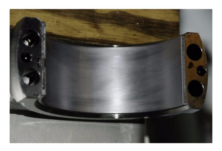
Crankshaft and connecting rod bearings are made using specific metals, copper, tin and lead. Which metal, and the quantities in which they appear in a report, are an indicator of the severity of wear. The bearing shown here (top) is severely damaged, the result of oil starvation caused by a clogged oil gallery. By comparison this bearing (above) is healthy, it is wearing normally.
