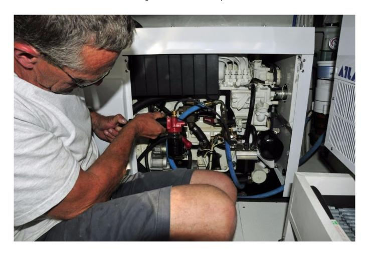
Properly drawing oil samples, here a boat owner carries out this task using a vacuum pump and dip tube, is of paramount importance where oil analysis accuracy is concerned.
