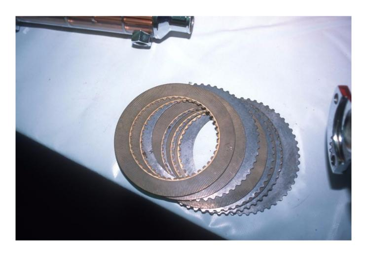
Many hydraulic transmission rely on sintered bronze clutch plates, which, under normal conditions, generate copper particulates, which in turn are identified in an oil analysis. Typically, this is, provided the quantity is normal based on the lube time, no cause for alarm.
