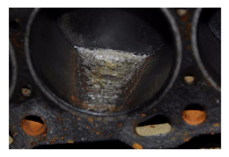
Seawater leaking into cylinders, often from a defective or improperly-designed exhaust system, frequently leads to catastrophic damage. It also can show up in oil analysis reports long before the damage is serious or irreparable.
