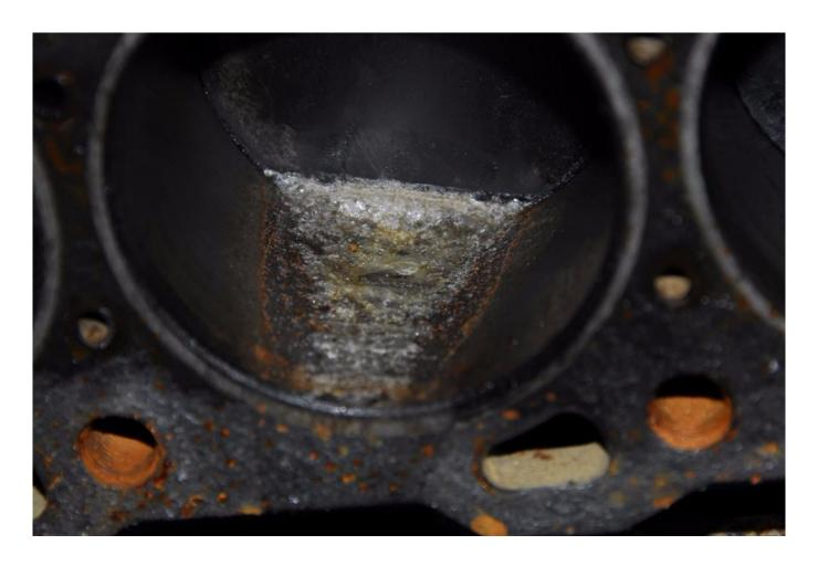
Seawater leaking into cylinders, often from a defective or improperly-designed exhaust system, frequently leads to catastrophic damage. It also can show up in oil analysis reports long before the damage is serious or irreparable.
