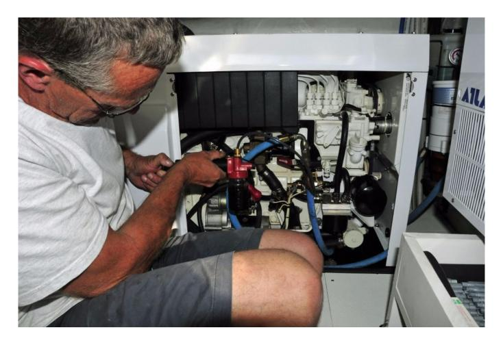
Properly drawing oil samples, here a boat owner carries out this task using a vacuum pump and dip tube, is of paramount importance where oil analysis accuracy is concerned.
