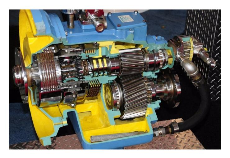
Transmissions are every bit as complex as engines, and while they don't suffer from exhaust byproduct contamination issues, they can develop faults that are identifiable in an oil analysis report.
