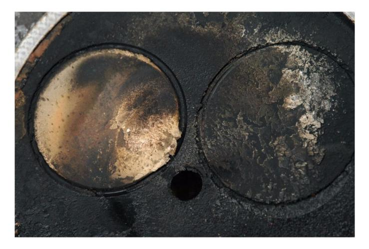
This engine experienced a head gasket failure, which allowed small amounts of coolant to leak into the combustion chamber, evidenced by this tan-colored accumulation on an exhaust valve. This sort of fault is often quickly identifiable using oil analysis, long before symptoms, or damage, manifest themselves.
