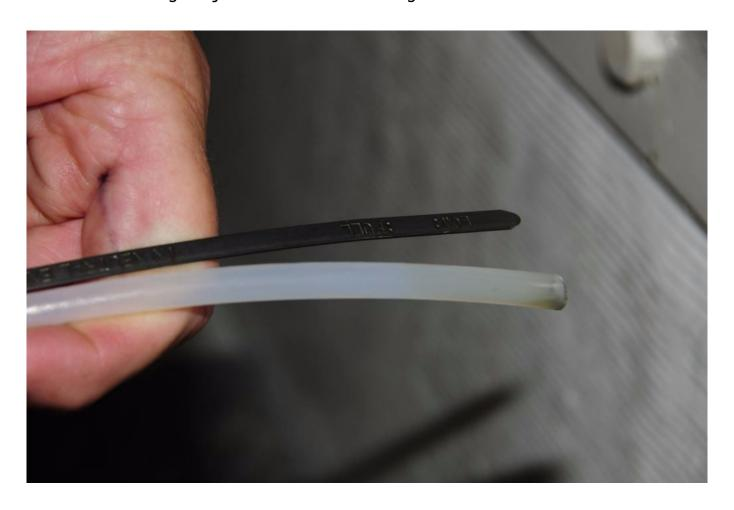
Overly long sample tubes can lead to "dredging", wherein the sample is contaminated with years' worth of oil sump accumulation. The results of such samples are of little use.
