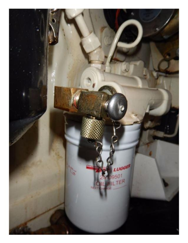
An oil sampling valve enables samples to be taken from an operating machine, yielding the most representative type of sample, without the need for a vacuum pump or tubing.
