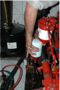
Vertical, opening facing down, and horizontal oil filters present a challenge when changing. Be prepared with plenty of rags and oil absorbant pads.
