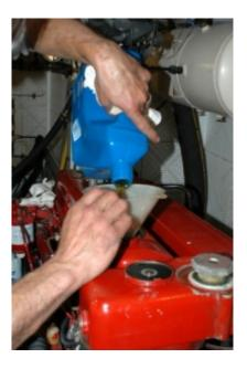
Once again, when adding oil, observe absolute cleanliness. Be certain no debris, dust or dirt are on top of the oil container, around the fill cap or in the funnel.
