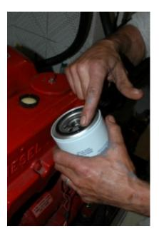
Lubricate the gasket of the new filter with clean oil. If the filter installs vertically, opening side up that is, then precharge the filter with clean oil. When lubricating the gasket or pre-charging the filter, observe absolute cleanliness, any debris that makes its way into the filter will enter the engine without filtration.
