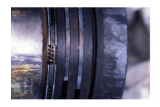
Combustion byproduct gasses bypass the piston rings (this is known as blow by), seen here, and make there way into the crankcase, where they contaminate the lubricating oil. Some blowby is normal, excessive blow by, on the other hand is undesirable and indicative of other problems.
