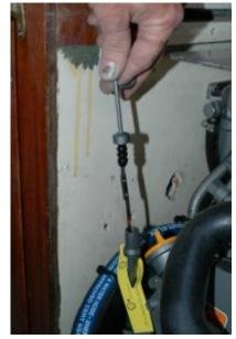
registers FULL on the dipstick. Do not overfill, if you do the crankshaft may collide with the oil in the pan. When it does so it's as if it's hitting a solid mass (ever do a bellyflop from a diving board? If you have you know what the crankshaft feels like when it hits the oil at hundreds and thousands of times a minute. This may lead to crankshaft/bearing damage or oil aeration, which in turn may cause erratic running characteristics, lubrication starvation or accelerated oil oxidation.
