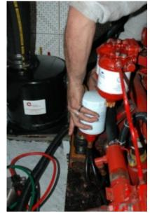
Vertical, opening facing down, and horizontal oil filters present a challenge when changing. Be prepared with plenty of rags and oil absorbant pads.
