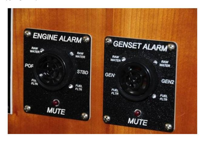
Onboard "alarms"fall into a variety of categories and levels of criticality. The alarm panels shown here monitor both exhaust system temperature as well as the accumulation of water in fuel filters, for propulsion engines and generators aboard this vessel. When the audible alarm sounds, an accompanying light quickly alerts the vessel operator as to which component is in need of attention.
