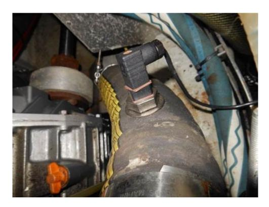
Exhaust alarm sensors that must penetrate the hose, where they operate in the exhaust gas and water stream, live an especially arduous, and failure prone life.
