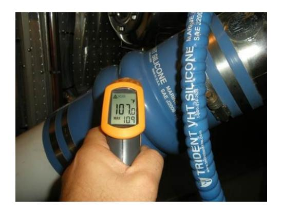
This exhaust system is operating normally. While the threshold temperature is 200°F, typically, well designed wet exhaust systems operate below 150°F. Most water cooled exhaust alarms trigger at approximately 165°F.
