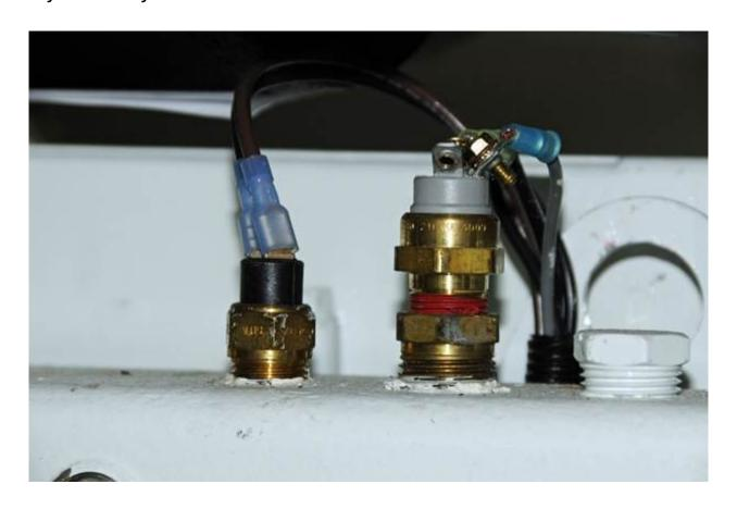
In many cases, if engine alarms don't exist, senders must be added. Typically, this is not especially difficult; however, consideration must be given to their physical security and the potential for vibration-induced failure.
