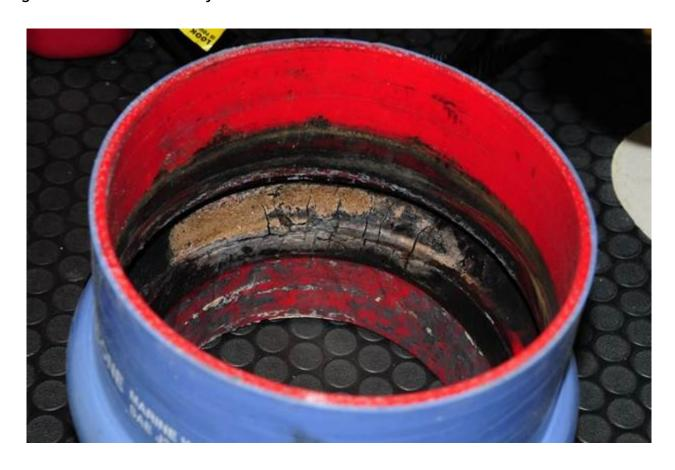
This exhaust hose has suffered damage as a result of exhaust system overheating. The engine itself did not overheat and therefore no alarm sounded, the vessel was not equipped with an exhaust temperature alarm.
