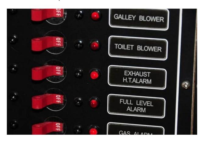
Exhaust system alarms should be "armed" and ready to sound in the event of an overheat, whenever an engine is running.
