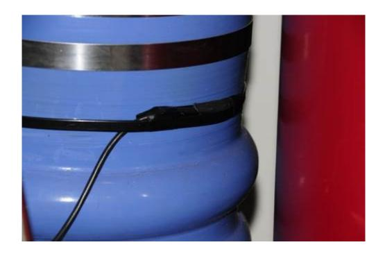
Surface mount alarm sensors or thermistors, like the one shown here from Borel Systems, offer two attributes, they respond very quickly to temperature change, and they don't need to be exposed directly to exhaust gasses.
