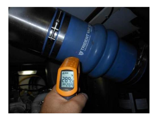
This exhaust hose is overheating. Often, and counterintuitively, water-cooled exhaust systems will overheat when the vessel is operating at low rather than high speed; at low speed less water is pumped into the exhaust system, often leaving the upper portion of hoses dry. The threshold for all portions of a water cooled exhaust system is 200°F.
