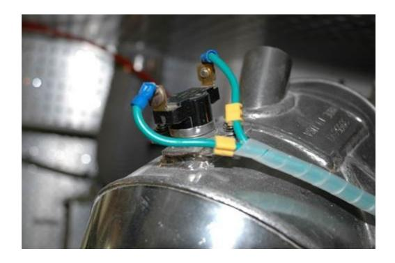
Exhaust temperature alarms are especially valuable, and required for compliance with American Boat and Yacht Council guidelines; the one shown above monitors temperature of the metallic mixing nozzle. Because of its mass this type of alarm can be slow to react.
