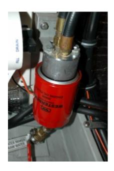
This oil filter has been remotely mounted, greatly improving serviceability. The builder has chosen to stay with the OEM filter.
