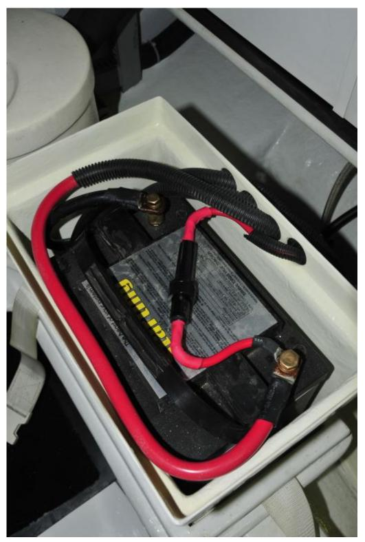
The small gauge wire shown here, likely for a charging circuit, is properly over-current protected with an in-line fuse.
