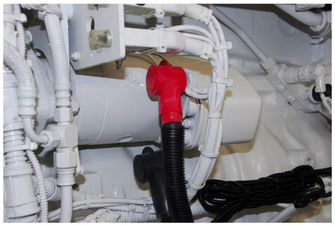
Cranking or starter circuits are exempt from the ABYC overcurrent protection guidelines. However, the positive or "ungrounded" conductor must not make contact with any part of the engine. The installation shown here is compliant.
