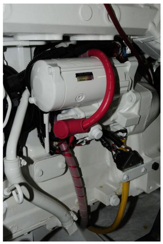
This starter cable routing represents a clear violation of ABYC Standards; positive starter cables must not make contact with any part of the engine. If it were to chafe to the starter or block, establishing a short-circuit, it would rapidly overheat, and possibly lead to a fire.
