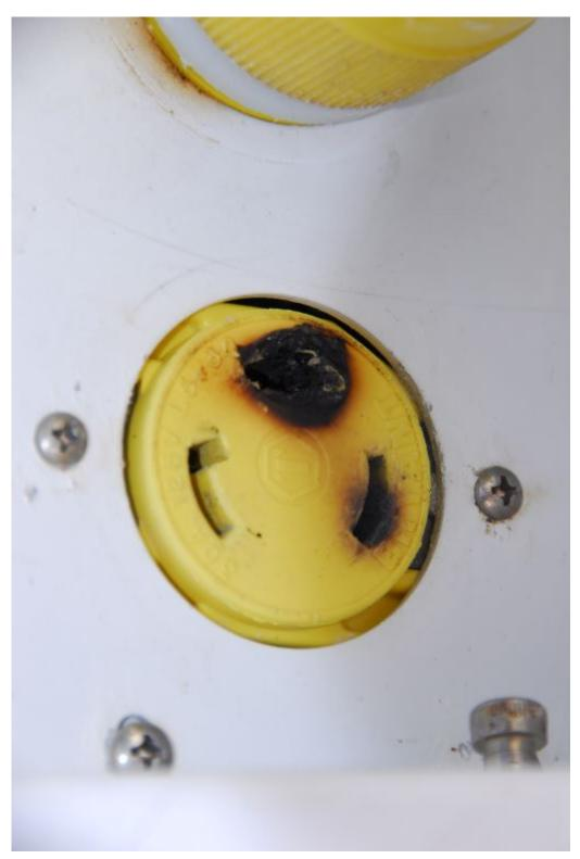
Contrary to popular belief, over-current protection will not prevent high resistance scenarios like the one shown here. High resistance, which creates heat, is indistinguishable from other normal loads like space heaters, ranges and hair dryers.
