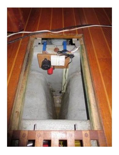
The high water alarm (white box), 9v battery operated, with sensor at end of black wire going down deep into bilge for early warning, is visible in this image. Also shown is a buzzer (black)indicating electric bilge pump activation and a secondary sensor (orange) to detect propane fumes.
