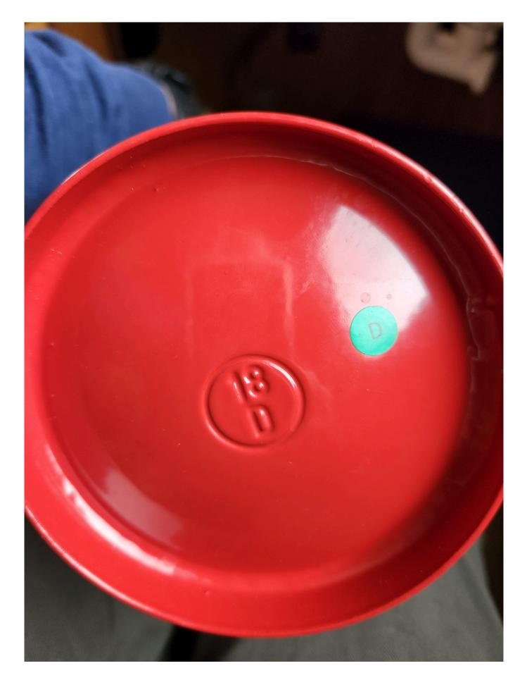
Most disposable fire extinguisher bottles are stamped with the date of manufacture, if it's only two numbers, like the one
