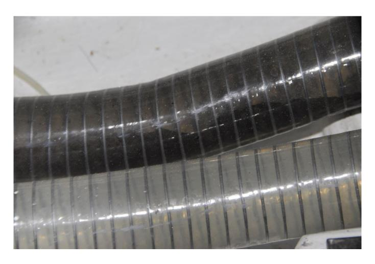
The upper hose is contaminated with biological growth, evidenced by its darkened color. Growth of this sort can lead to foul smelling and tasting water, as well as illness for those consuming it.
