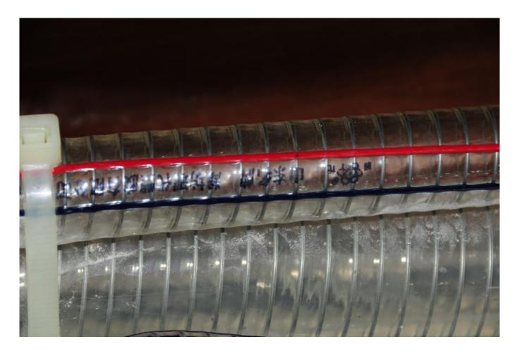
Hose that lacks a legible designation for potable water use is not suitable for this application. Insist that your yard or builder use hoses that clearly specify that they are for potable water applications.
