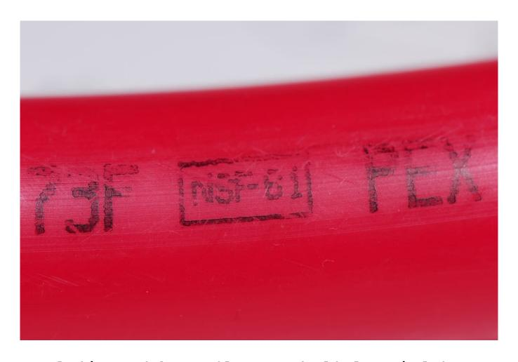
Plumbing used for potable water should always include a designation ensuring it is suitable for the application, such as 'NSF-61' shown here.
