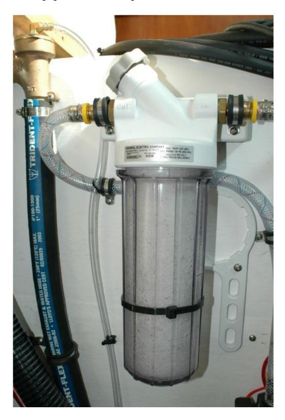
Whole vessel filters may rely on a clear bowl. This is acceptable for use inside the vessel, however, avoid using these on the dock for pre-filtration as they will support
