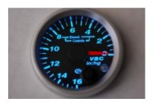
Electronic, "differential" vacuum gauges will indicate vacuum across the filter alone, providing a clear indication of the element's condition.
