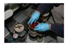
Replacing the element in a Racor Turbine series primary filter is straightforward.
