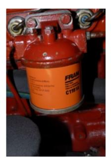
On-engine secondary filters, on the other hand, particularly those of the, "sandwich" variety can be especially challenging to replace.
