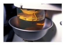
Primary filters are capable of capturing and holding a tramendous amount of debris and water.
