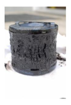
Although the vacuum reading was in the teens, the engine served by this primary (10 micron) filter element continued to operate, which is indicative of just how valuable these filters are when it comes to capturing and holding debris and contamination.
