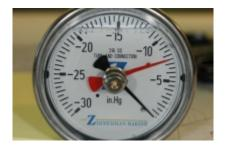
Recording vacuum gauges such as the one shown here are valuable tools in that they record the highest vacuum experienced by the filter at any time until reset.
