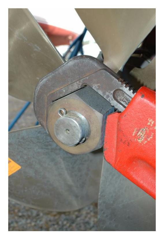
A smooth jaw wrench, shown here, is designed for turning hex nuts, while pipe wrenches rely on sharp, hardened teeth, which are designed to turn pipes by cutting into them. Pipe wrenches should never be used on hex nuts, doing so invariably leads to damage.
