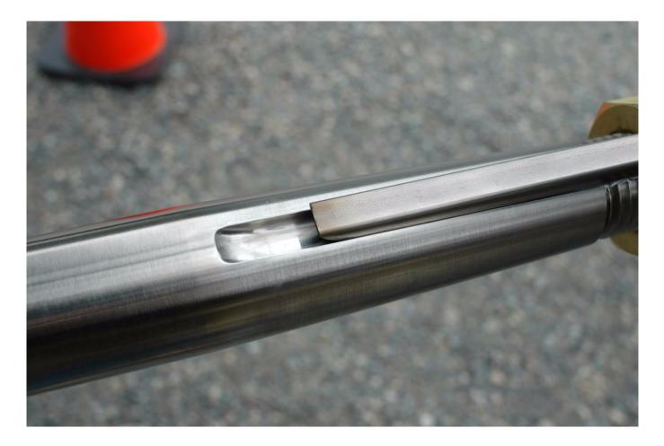
Keys should fit snugly into keyways, not too loose and not too tight. If the key is too loose, the propeller can move independently of the shaft, which in turn will lead to keyway damage.
