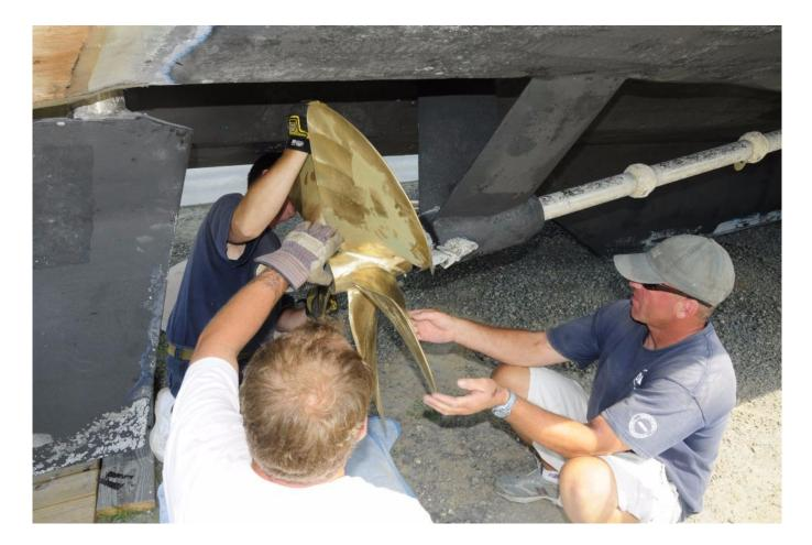
The lapping process involves rotating the propeller clockwise and counter-clockwise several times on the shaft, then checking the condition of the machinist's dye to determine the level of interface between the two.
