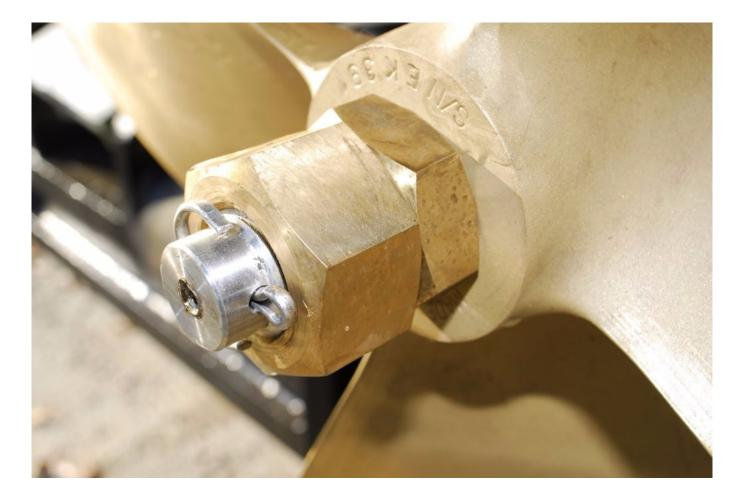
Bronze propeller nuts are self-lubricating and as such less prone to thread galling. The nuts shown here are installed in the correct order, half height nut first, then full height nut.
