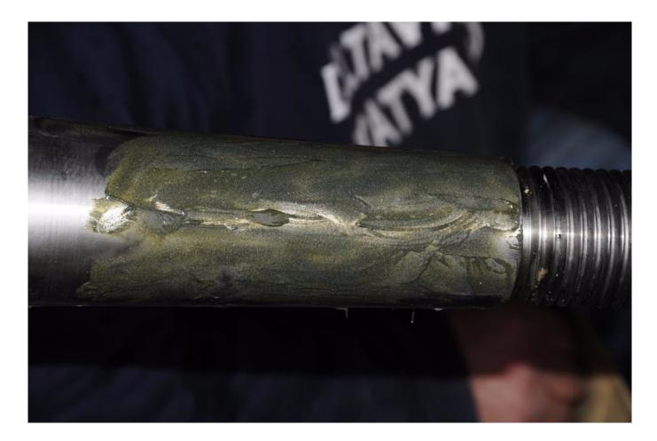
Lapping compound, shown here having been applied to a shaft taper, has the consistency of we sand. It removes material from the prop bore, allowing a custom fit between bore and shat taper.
