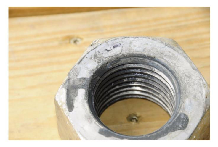
Stainless steel nuts are susceptible to galling, a phenomenon wherein the threads overheat and metal is moved from one thread to the other, when installed on a stainless steel alloy propeller shaft. This can be avoided by lightly lubricating the threads.
