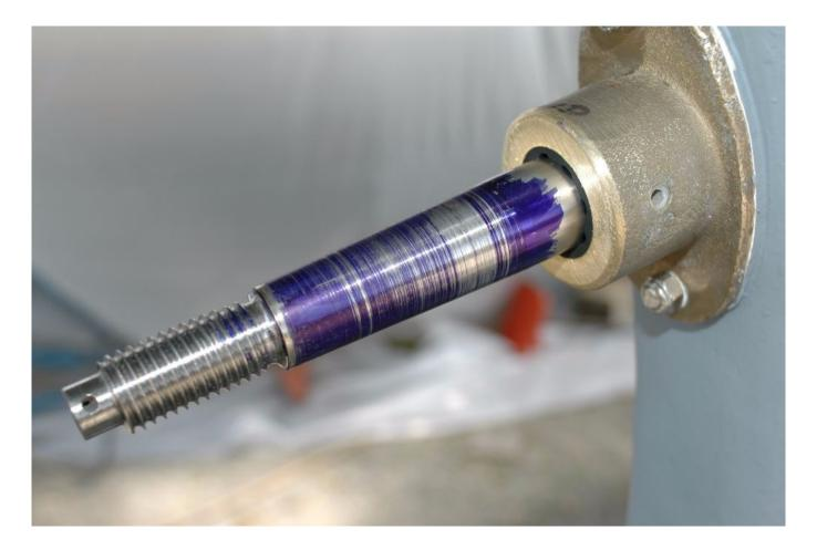
Machinists dye, typically blue or purple, acts as an indicator, determining where the shaft and prop are making contact. The goal is to achieve at 90% contact, which means 90% Of the dye is removed after successful lapping.
