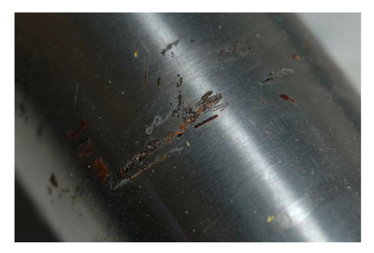
Inspect shaft tapers for any signs of corrosion, pitting, scoring or any irregularity. Pitting, shown here, would require repair or replacement of the shaft.
