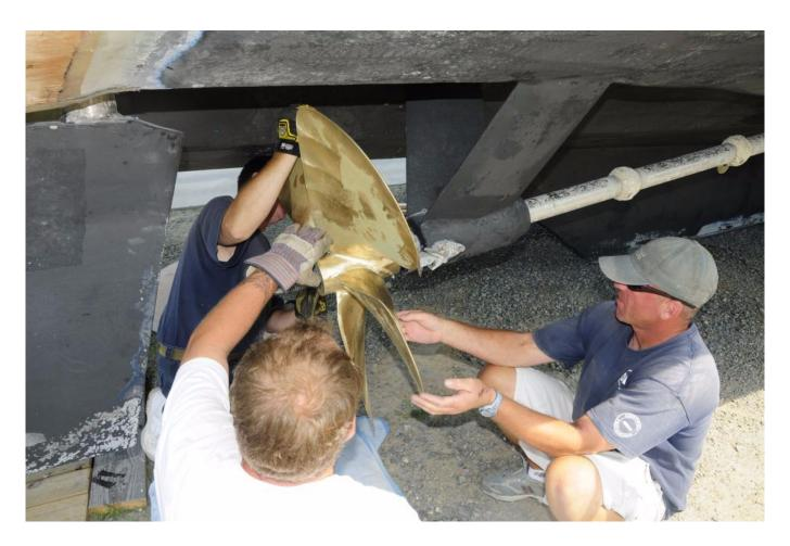
The lapping process involves rotating the propeller clockwise and counter-clockwise several times on the shaft, then checking the condition of the machinist's dye to determine the level of interface between the two.
