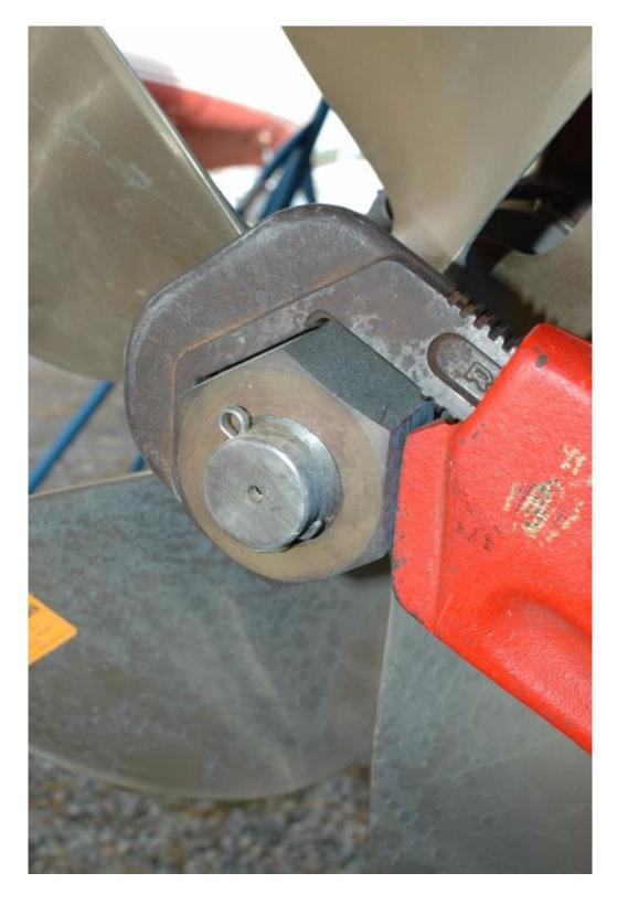
A smooth jaw wrench, shown here, is designed for turning hex nuts, while pipe wrenches rely on sharp, hardened teeth, which are designed to turn pipes by cutting into them. Pipe wrenches should never be used on hex nuts, doing so invariably leads to damage.
