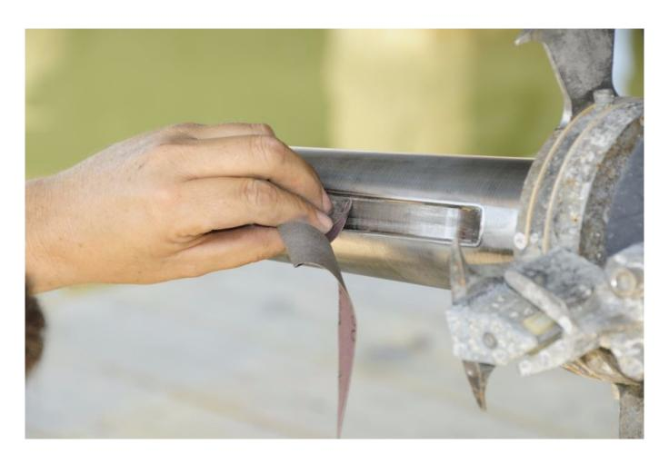
Keyways should be clean and free of debris or scale, to ensure the key fits properly, and avoids binding of the propeller during installation.
