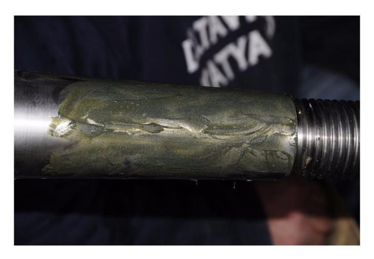
Lapping compound, shown here having been applied to a shaft taper, has the consistency of we sand. It removes material from the prop bore, allowing a custom fit between bore and shat taper.
