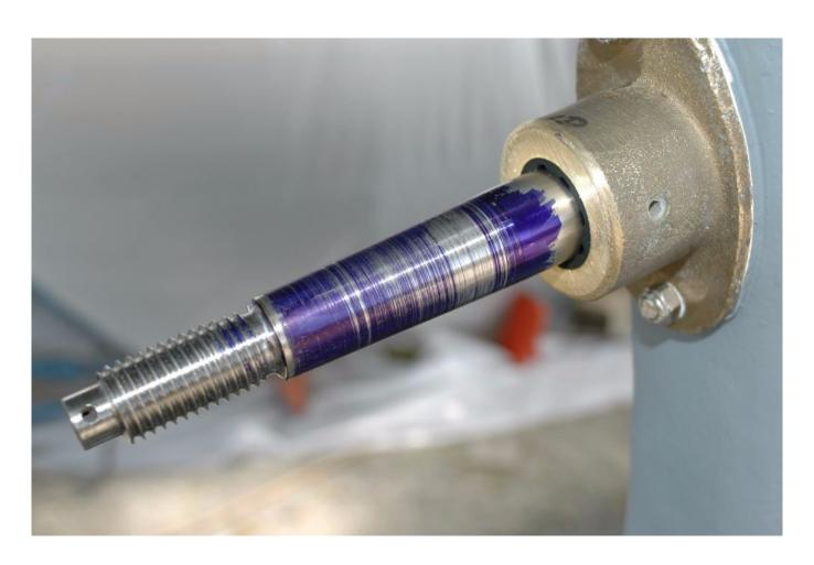
Machinists dye, typically blue or purple, acts as an indicator, determining where the shaft and prop are making contact. The goal is to achieve at 90% contact, which means 90% Of the dye is removed after successful lapping.
