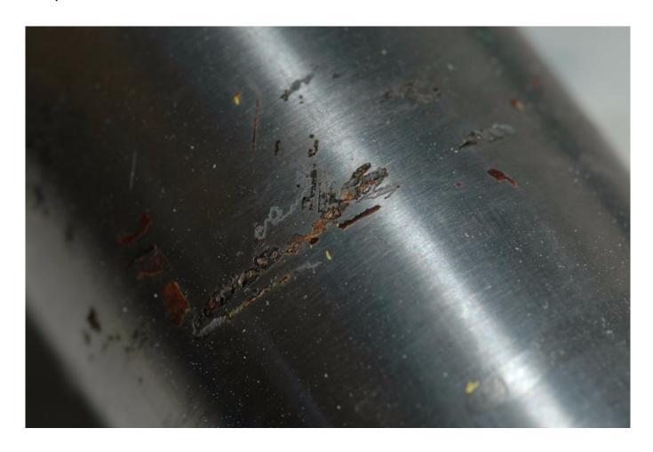
Inspect shaft tapers for any signs of corrosion, pitting, scoring or any irregularity. Pitting, shown here, would require repair or replacement of the shaft.
