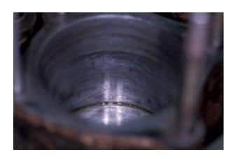
Properly broken-in cylinder walls. Note the crosshatching remains intact.
