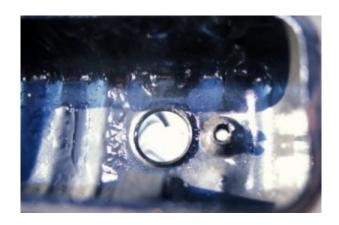
When there is sludge inside your valve cover, there is blow by occuring in your engine. It's a result of a mixing of oil and water vapor, the latter is contained in exhaust gasses.
