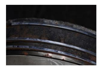
The rust deposited adjacent to these piston rings clearly
