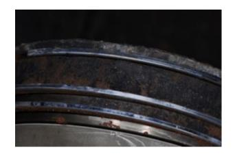
The rust deposited adjacent to these piston rings clearly
