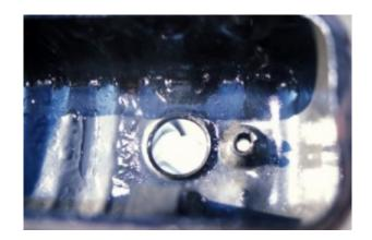
When there is sludge inside your valve cover, there is blow by occuring in your engine. It's a result of a mixing of oil and water vapor, the latter is contained in exhaust gasses.
