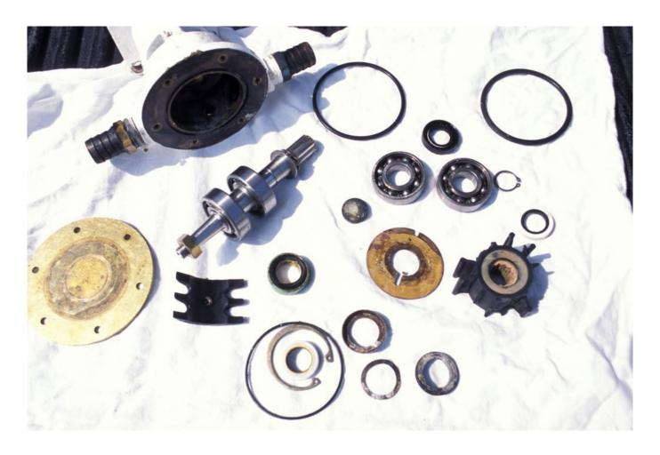
The average raw water pump contains many pieces, making field rebuilding more than a simple affair. A press is sometimes needed to remove bearings.
