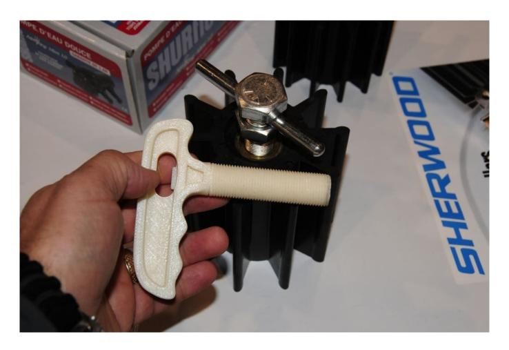
For impellers that are equipped with threads, jacking screws can be used for removal. These are especially valuable where clearance does not allow for an impeller puller.
