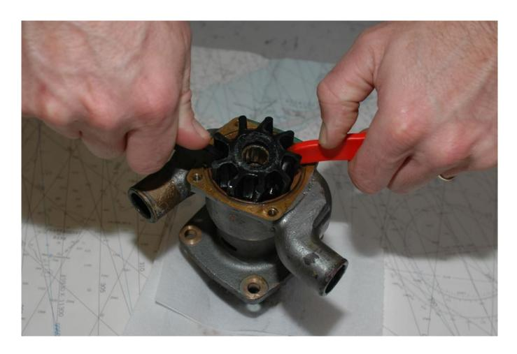
Never use a screw driver or other hard object to pry out an impeller. Plastic pry bars, on the other hand, may be used without concern for causing damage.
