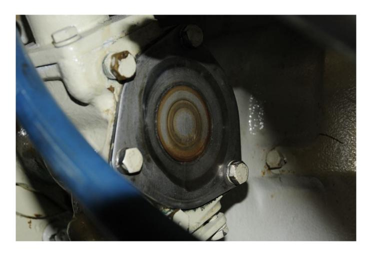
Most pump cover plates can be turned over, as this one has, for a second life provided there is no, or little, embossed lettering on the surface against which the impeller will turn.
