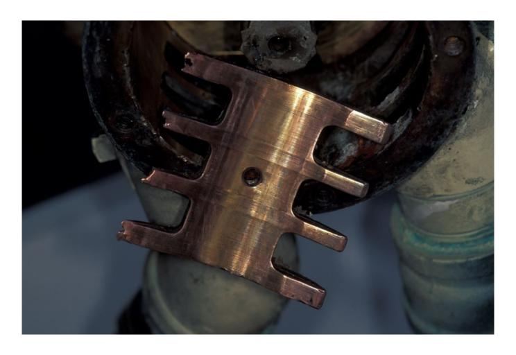
Determining the wear level of a cover plate and cam, particularly the latter, can be difficult until compared to replacements.
