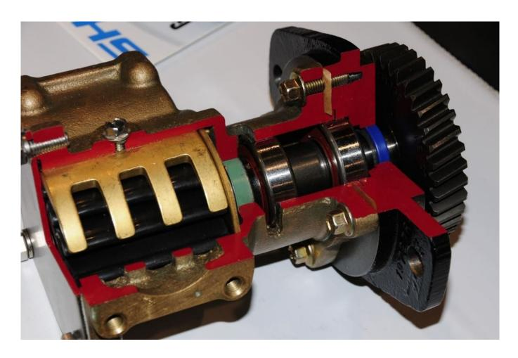
Bearing races, the silver rings, along with the cam (as well as the retainer screw and washer), fork-like object on the left, can be seen in this cut-away of a pump. Most geardriven pumps like this utilize a void between the oil and raw water seals, which includes a telltale or weep hole on the bottom side, which will allow oil or water to exit if one of these seals leaks, alerting the user to a problem, and preventing water from entering the crankcase
