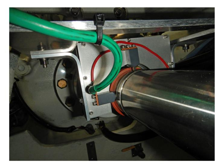
Silver slip ring shaft brushes are capable of meeting the 1 ohm resistance requirement, which is required for cathodically protecting shafts and props with remote anodes.
