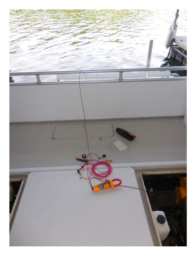
Corrosion analysis underway; testing should take place in still water, initially with shore cord unplugged, and then plugged in. If the readings change after reconnecting the shore cord, a problem exists.
