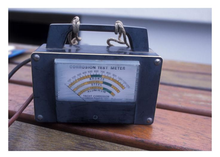
Proprietary corrosion monitors, which are simply graduated analogue ohm meters, are available and easy to use. Beware: This legacy meter shows a protected range for aluminum that is
