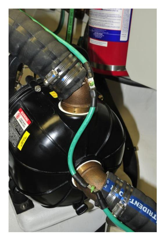
Bonding otherwise isolated, fully internal raw water plumbing components, while not harmful, will afford them no protection from galvanic corrosion. Bonding may provide protection from stray current corrosion if the plumbing is submerged in bilge water.
