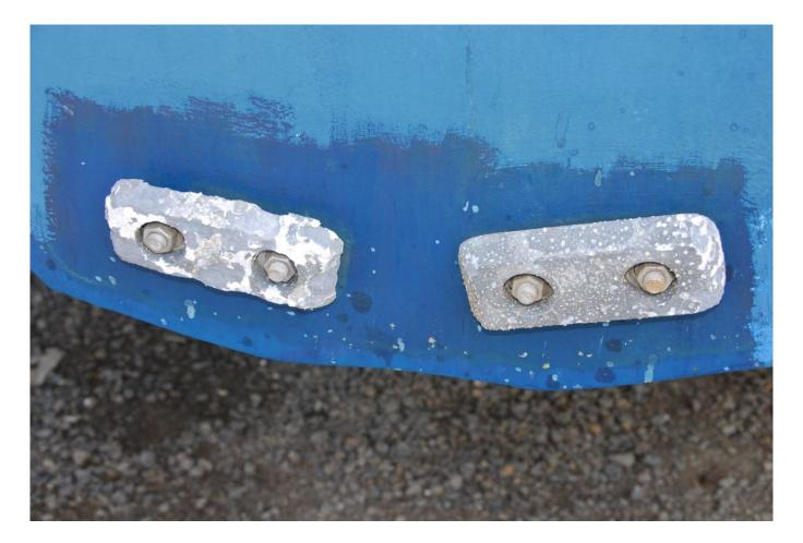
An indication of trouble; like anodes that are connected to a common bonding system, and are adjacent to each other, should
