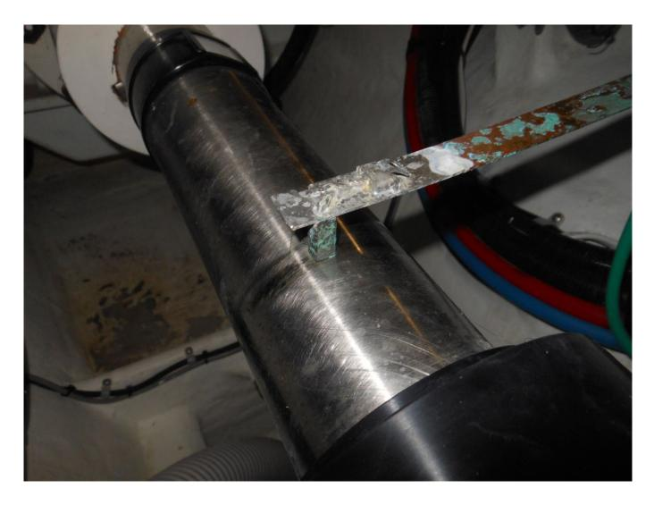
Conventional 'wand and carbon brush' style shaft brushes, are incapable of meeting the sub one ohm resistance threshold, required for cathodic protection systems.
