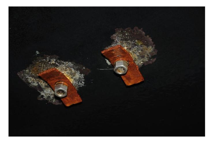
Neglecting anode replacement can be a costly error. Here, all that's left of this anode is its embedded plates, all of its sacrificial metal is long gone.
