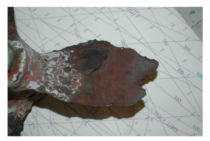
Stray current corrosion is vicious and rapid, it can destroy a propeller like this in a matter of days. While sacrificial anodes may do little to prevent it, a reference cell can be used to help identify its presence and the source.
