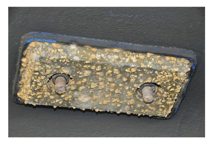
Zinc anodes used in fresh water develop a coating, which renders them useless. If the vessel returns to seawater, the coating can be removed with a non-metallic, stiff bristle brush.
