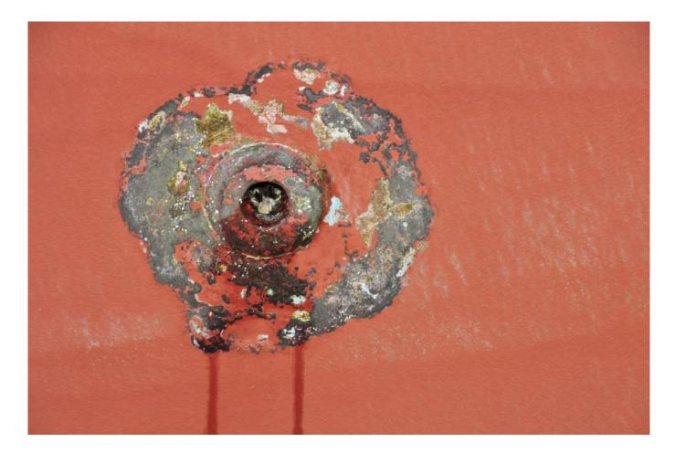
Paint failure around bonded/protected underwater metals is often an indication of over-protection. On fiberglass vessels this is only harmful to the paint and can be mitigated with an epoxy primer.
