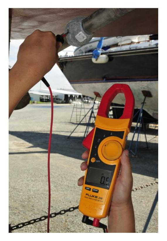
The resistance between an anode, and the metal it's
