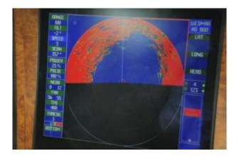
Having the ability to confidently "see" what is happening below and ahead of your vessel is a stress-reducer when cruising in unfamiliar, or poorly charted waters. This "searchlight" sonar enables this vessel to enter poorly charted, infrequently visited inlets and bays, which is part of the attraction. Charts for many remote areas often rely on surveys made by early explorers and whalers, with lead line and sextant.
