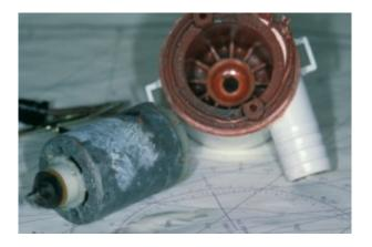
And this could have been the culprit, the failed bilge pump motor was leaking DC current directly into the bilge water which was in contact with an un-bonded through hull, and through the water and to the prop.
