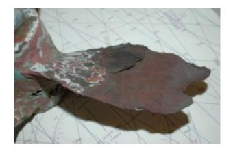
This propeller blade has been destroyed by stray DC current corrosion from a damaged bilge pump. While it may have occurred in a marina, it was not the direct result of AC or shore power current.
