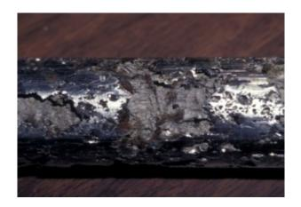
This stainless steel prop shaft suffered extreme corrosion and was clearly condemned. This is very likely a case of stray current corrosion, which is nearly always associated with DC rather than AC or shore power current.
