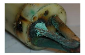
Beneath the rubber boot, this 50-amp shore power cord is severely corroded, probably as a result of it falling into the water. The insulation of one of the hot or energized wires is almost entirely melted away and is nearly touching the green grounding wire.
