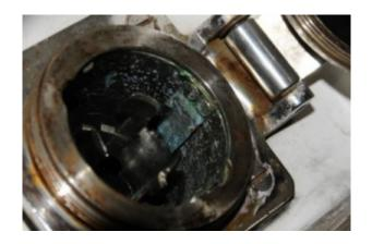
The green tab inside this 50-amp shore power connection should be bright metal. The tab is the ship's connection to shore ground and when it is corroded that connection is compromised, jeopardizing the safety of the crew.
