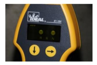
There are several useful tools you or a qualified marine electrician can use to diagnose faults within the AC system aboard your boat. This Ideal circuit tester shows an AC receptacle with a missing ground connection.
