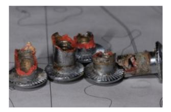
These fasteners are suffering from galvanic corrosion and specifically dezincification. They are chrome-plated brass, which has a high zinc content, and they are unsuitable for marine applications.
