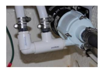
Conventional PVC plumbing is ill-suited for raw water use and should be avoided in locations where its failure will lead to flooding.
