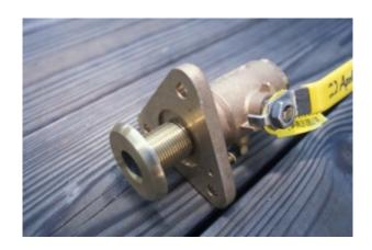
Through hull fittings and proper, flanged seacocks share the same thread type, NPS or straight.
