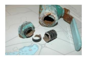
Don't make the brass mistake. Because of its susceptibility to dezincification, brass should never be used in any raw water plumbing application. True, zinc-free bronze, on the other hand is ideal.
