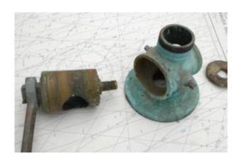
Traditional cone valves are extremely rugged and capable of being rebuilt over and over again.
