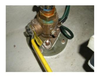
Proper seacock installations, like the one shown here, are robust and reliable. Many, on the other hand, fail to make the grade.
