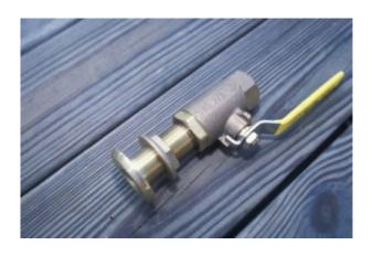
This arrangement, a ball valve mated to a through hull fitting often passes for a seacock, however, it's anything but.
