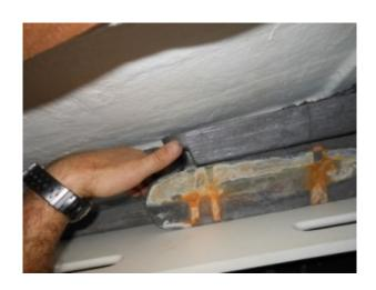
It's a common occurrence, lead ballast simply dropped into bilges or lockers, relying on gravity alone to keep it in place. Ballast should always be cribbed or otherwise secured in place to prevent any movement aboard any vessel. For blue water power vessels, this includes being heeled on their beam ends and for offshore sailing vessels, when inverted.
