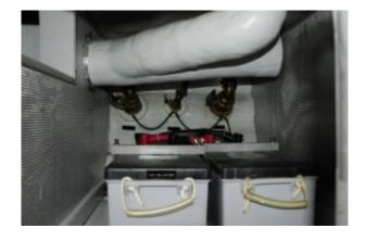
While it's not comfortable to reach over the batteries to access these at-the-waterline seacocks, they are easy to view
