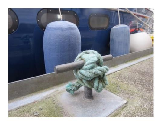
The proverbial Gordian knot...while it's doing the job it is sloppy and would be difficult to release quickly.
