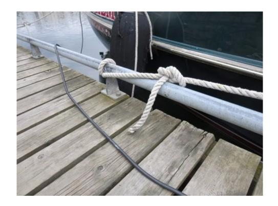
Hard to use a spliced loop here, however, as good as a bowline is, it can't be released under tension. Running the line around the pipe and back to the vessel's cleat would make more sense, although it would be susceptible to chafe if there's much movement.
