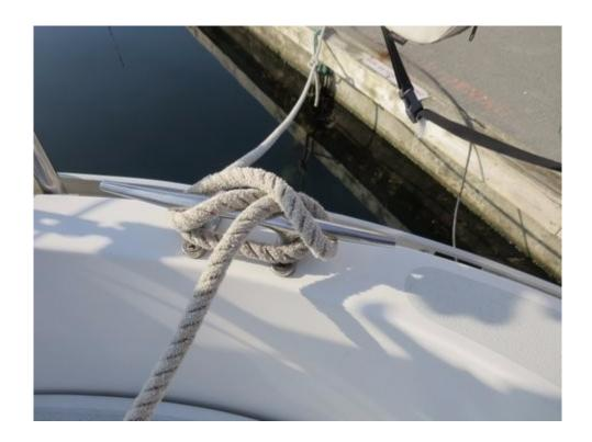
A proper cleat hitch, note the last bend, the two lines are parallel. It's easy and safe to surge a few inches or release. This is how cleats were designed to be used.
