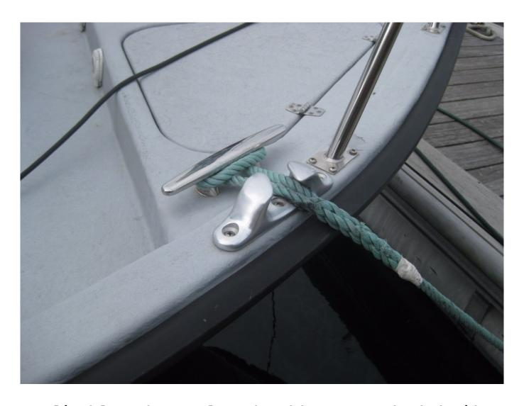
Spliced loops have a place aboard but not on the dock side cleat unless you are willing to abandon or cut the line.
