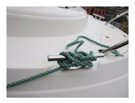
Hitching every turn is not proper cleat etiquette, while secure, it makes a quick release impossible.
