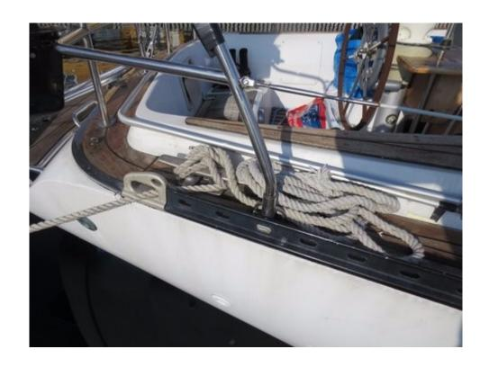
A good try, but the half hitch is piled on rather than laid alongside and will jam under load.
