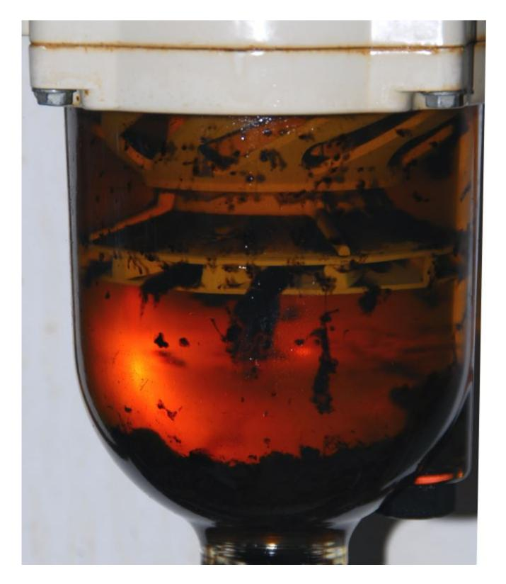
The dirt and water holding capacity of Turbine filters carries with it near legendary status. The engines served by the filters shown here continued to operate without issue.
