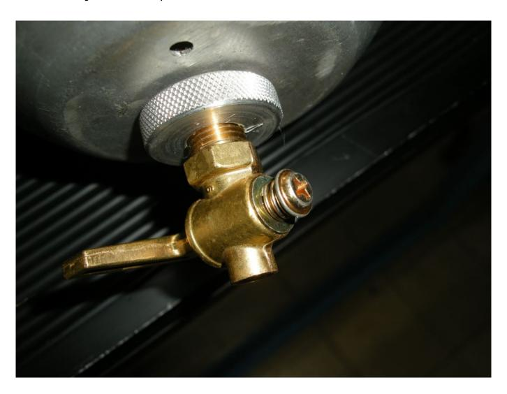
This drain lacks ABYC compliance for several reasons, it relies on a spring-tensioned seal (the spring is mild steel, which can rust and break), it turns through 360 degrees, and it lacks a pipe plug to prevent spills.
