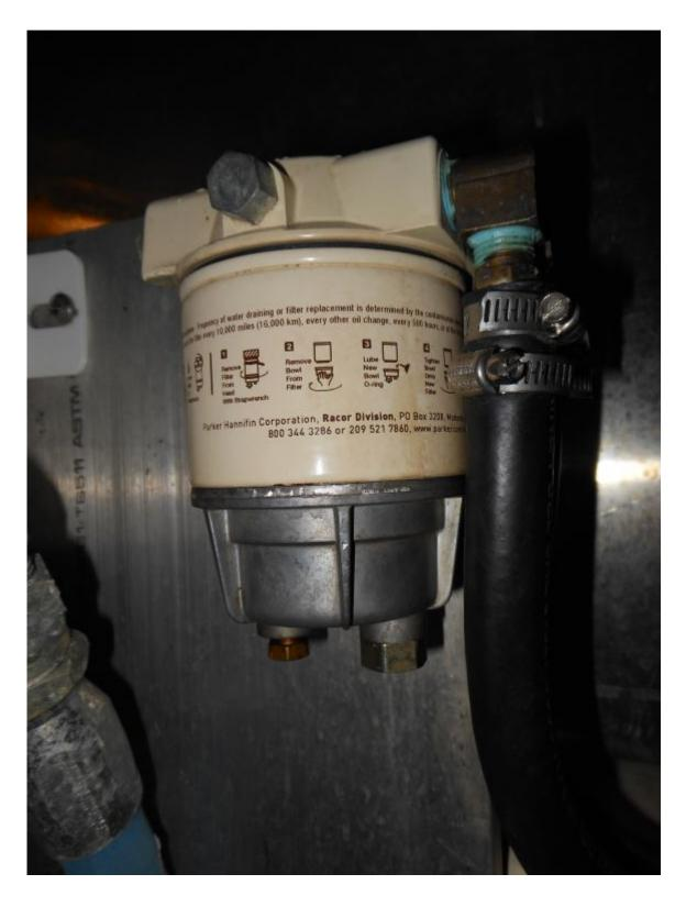
Smaller, non-turbine series filters may meet the fuel flow needs of generators and smaller propulsion engines, however, they are cumbersome to service, and in order to meet flame resistance standards they must forfeit their clear sight bowls, robbing them of one of their most valuable features.
