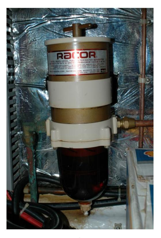
The lack of a heat shield and the candy-apple-colored label text belie this Racor Turbine Series primary filter's industrial, rather than marine origins.
