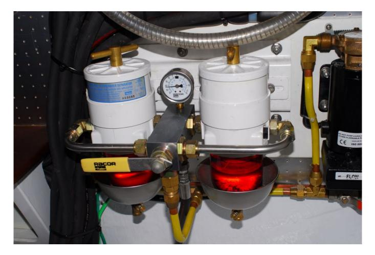
Racor Turbine Series filters offer users a host of advantageous features, and in the tandem arrangement like the
