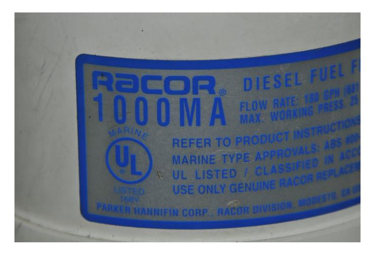
The blue font label on a MA Series Turbine filter denotes its compliance with ABYC and UL flame resistance standards.
