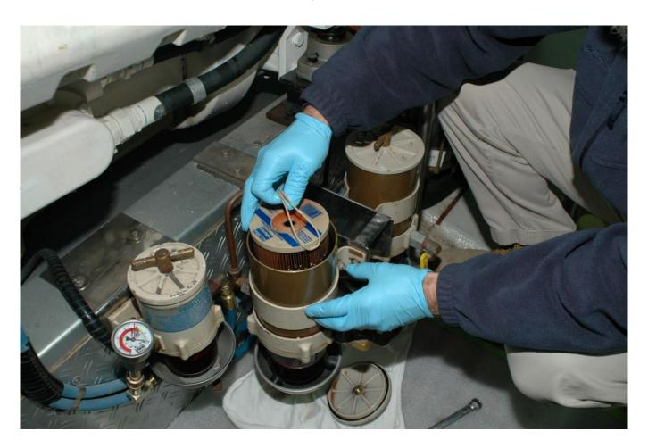
Few attributes of a fuel filter trump ease of service. When priming primary fuel filters of the sort shown here, be sure to do so only with the new filter element installed, thereby ensuring all fuel that leaves the filter body has passed through the element.
