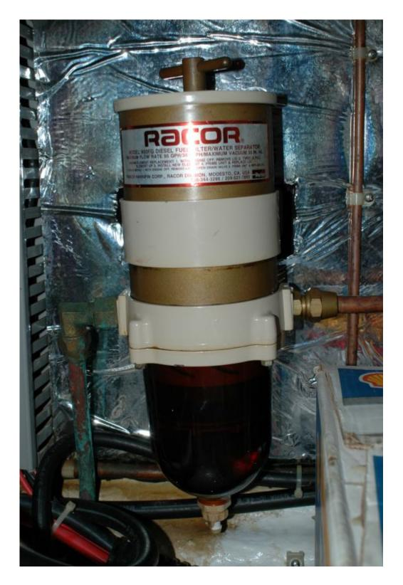
The lack of a heat shield and the candy-apple-colored label text belie this Racor Turbine Series primary filter's industrial, rather than marine origins.
