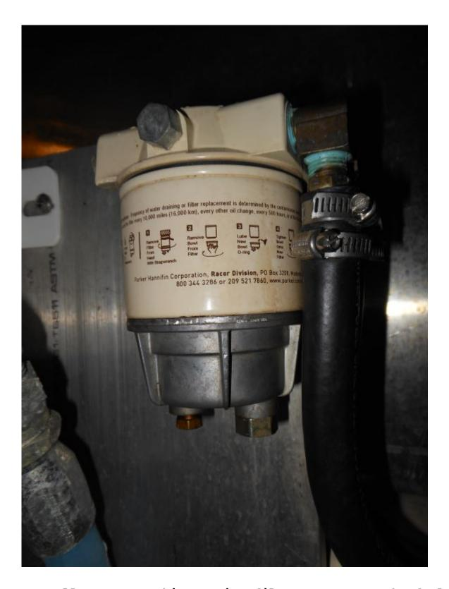
Smaller, non-turbine series filters may meet the fuel flow needs of generators and smaller propulsion engines, however, they are cumbersome to service, and in order to meet flame resistance standards they must forfeit their clear sight bowls, robbing them of one of their most valuable features.
