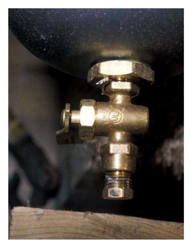
A UL Listed Marine drain valve must embody two features, a valve barrel whose fuel-tight seal does not rely on spring tension, and a handle that rotates through no more and no less than 90 degrees.
