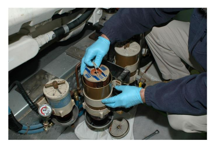
Few attributes of a fuel filter trump ease of service. When priming primary fuel filters of the sort shown here, be sure to do so only with the new filter element installed, thereby ensuring all fuel that leaves the filter body has passed through the element.
