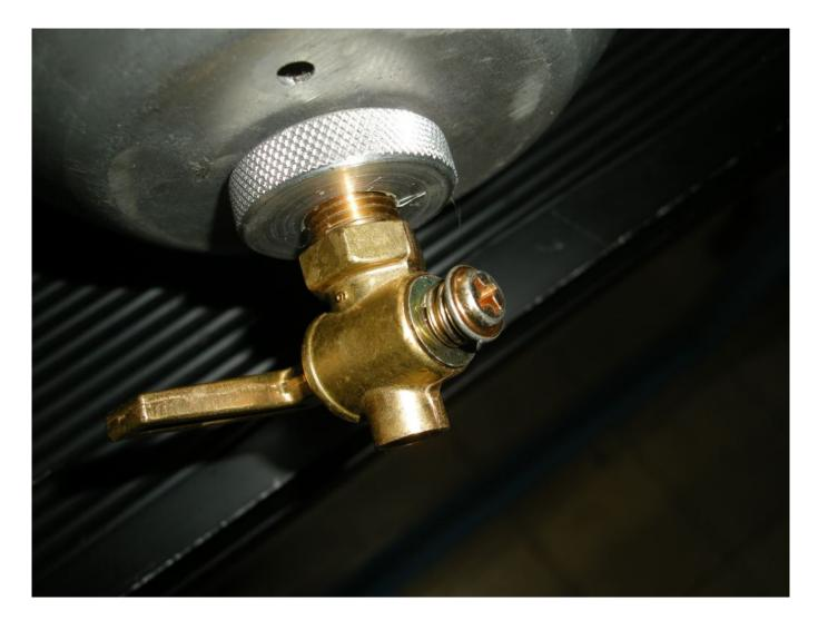
This drain lacks ABYC compliance for several reasons, it relies on a spring-tensioned seal (the spring is mild steel, which can rust and break), it turns through 360 degrees, and it lacks a pipe plug to prevent spills.
