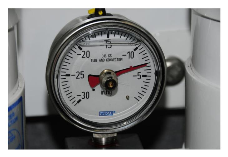
Without a vacuum gauge, you are flying blind… short of an engine shut-down, they are the only means by which filter condition can be determined. Running without one is tantamount to operating an engine with no coolant temperature, or oil pressure, gauges.
