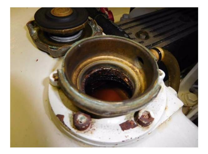
Not to be confused with a recovery tank or bottle, the expansion tank on closed cooling system engines is part of the pressurized cooling circuit; it's typically where the pressure cap is located.
